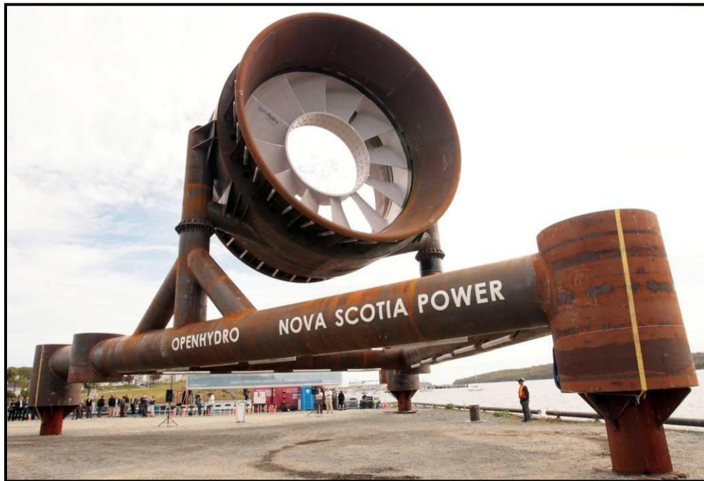
FIGURE 2-4 TRIAL ASSEMBLY OF 10 METER OPENHYDRO TURBINE AND SUBSEA BASE (DARTMOUTH, NOVA SCOTIA, CANADA)
