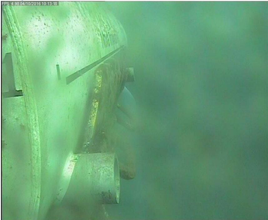
Figure 20 T1 SIDE: Biofouling begins to affect the camera view from October: 4_2016-10-04_10-05-32.mp4
