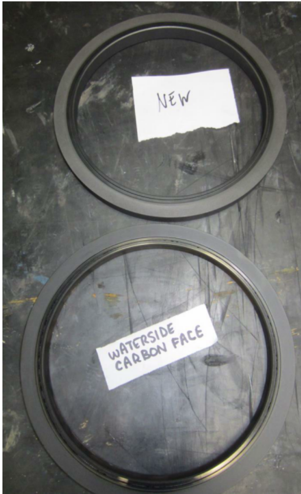
Figure 2.5 - Condition of Tested Outer Carbon Seal Face Compared to New Face
