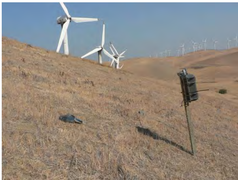
Photo 12. Example of camera setup for scavenger study. Right foreground: camera attached to angle-iron post. Left foreground: volitionally placed carcass of A11 (western scrub jay). Photo by K. S. Smallwood.
