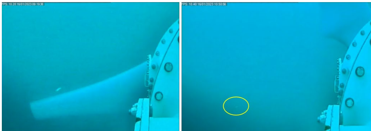
Figure 7-5 Stills from T6 camera containing fish identified by the model. In these clips the tide was running and the turbine blades were rotating. In the image on the right the fish which is small and passes quickly through the camera’s field of view is circled.
