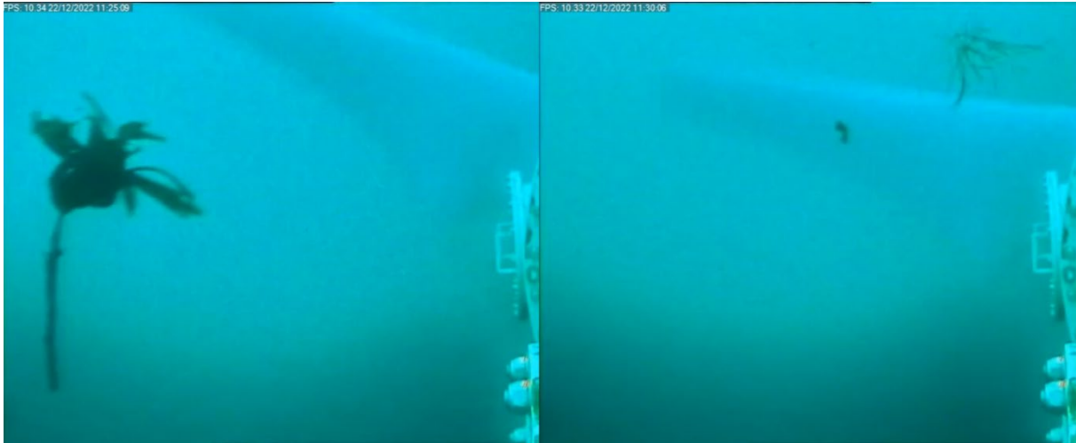
Figure 8-2 Examples of seaweed fragments which when viewed by manual reviewers can be confused with mobile species, particularly during peak flow speeds in Bluemull Sound.
