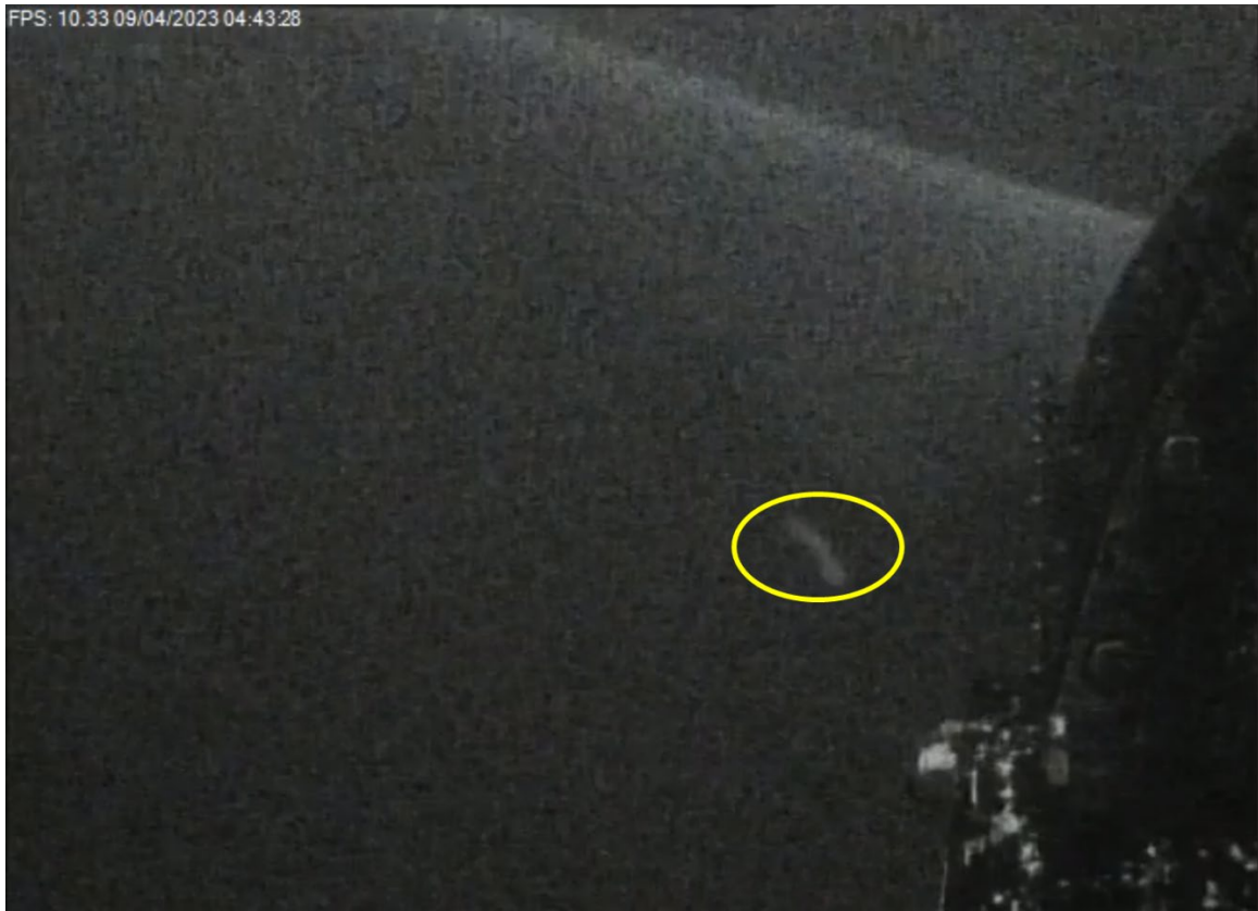
Figure 7-9 Still from T6 camera from 9 April 2023 showing a fish (circled in yellow) quickly passing the operating turbine on the maximum ebb tide. The object is only identifiable as a fish from observing the video at very slow speed.
