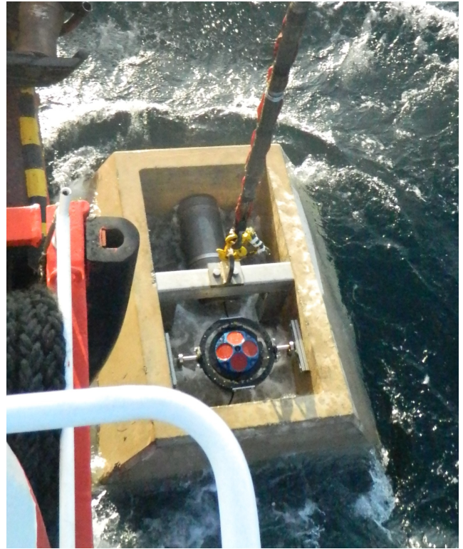
Fig. 7: D-ADP featuring custom damped gimbals set, concrete gravity mooring and custom anodised aluminium battery canister being lowered by the crew of KML's Severn Sea vessel.
