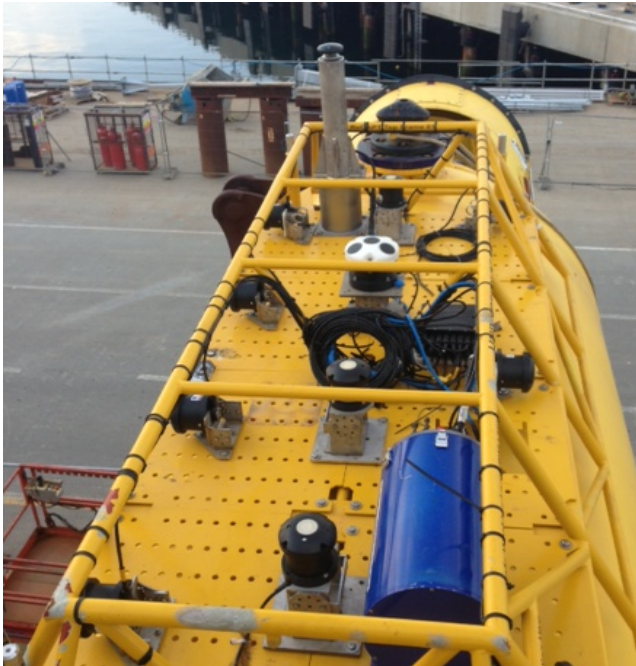
Fig. 4: Photograph of ESIP-1 taken from scissor lift platform showing instrumentation mounted atop the 1MW TEC at Hatston Quay, Kirkwall, Orkney prior to turbine deployment.
