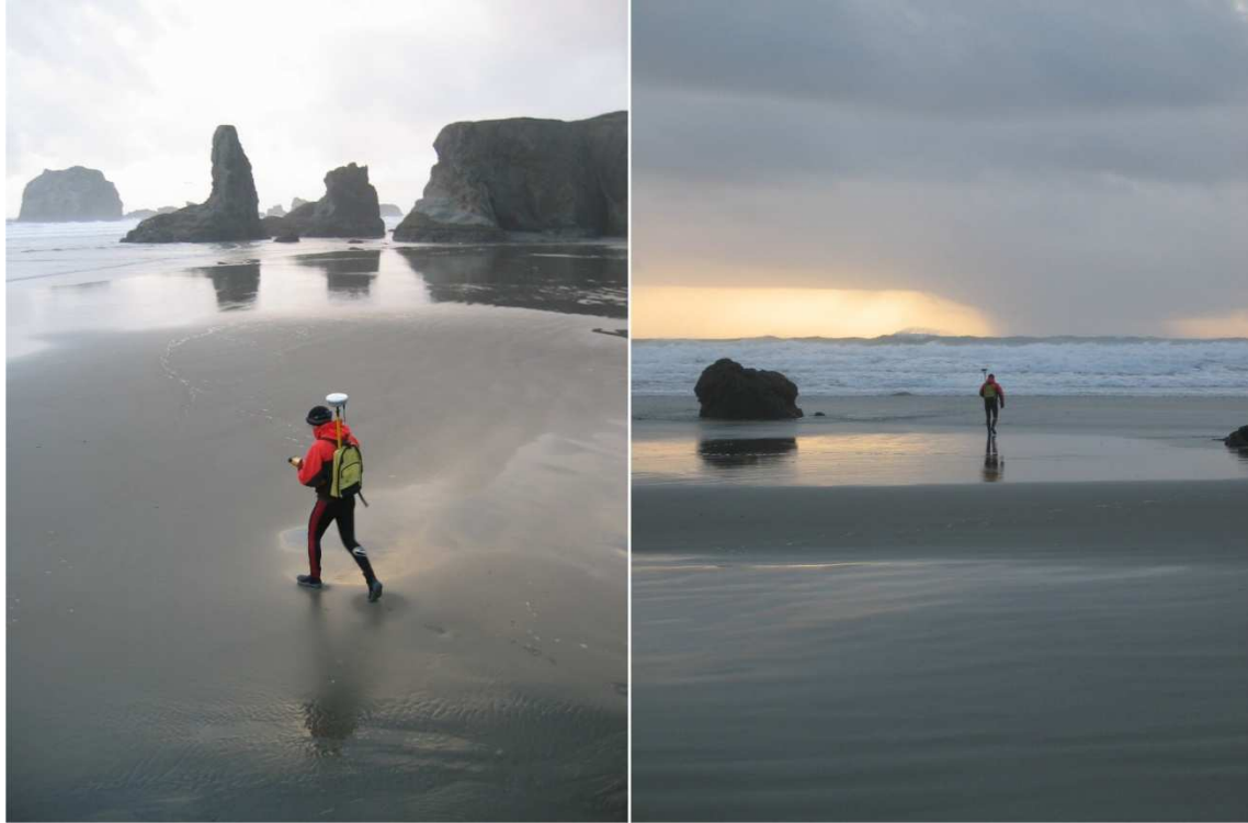
Figure A3 Surveying the morphology of the beach at Bandon using a Trimble 5800 ‘rover’ GPS.
