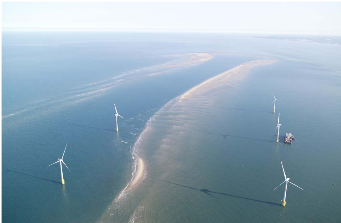
Plate 19. The subsidiary sand bar forming through the wind farm. Aerial photograph taken on 6 th July 2004 by Air Images Ltd. during a seal survey.
