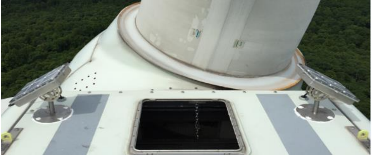
Figure 8. Photograph of two prototype UADs on the top of the nacelle, positioned near the rotor.
