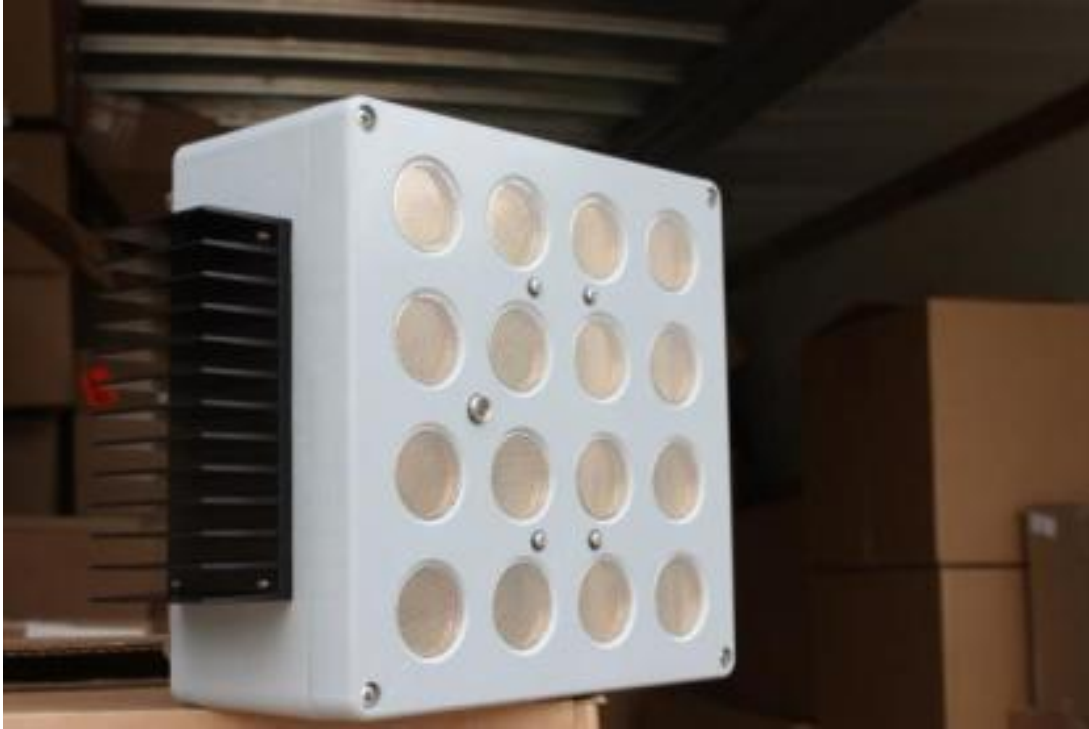
Figure 1. Photograph of the Deaton UAD with the 4x4 electrostatic transducer array. See Arnett et al. 2013 for more information on this device.
