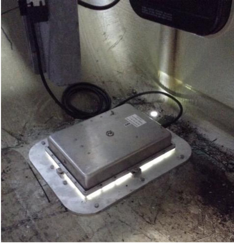
Figure 3. Photograph of an ultrasonic acoustic deterrent secured to the base of the nacelle.
