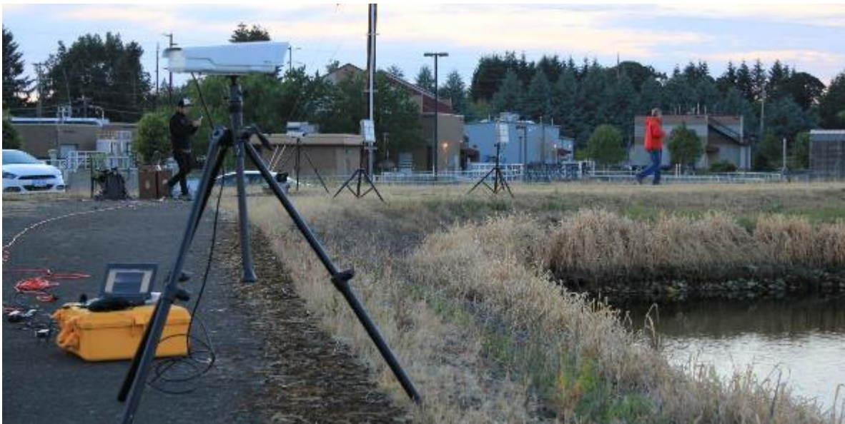
Figure 6. Positioning of a thermal camera (foreground) perpendicular to the location of the deterrents (background).
