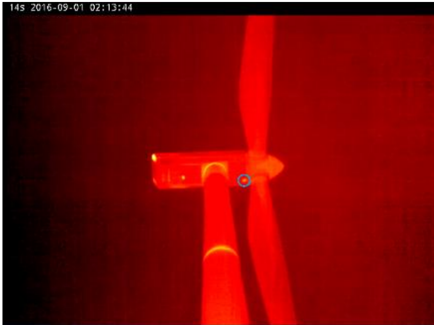
Figure 2. Screen shot from a thermal camera showing the nacelle reference point (blue circle) used to build 3D models of bat events.
