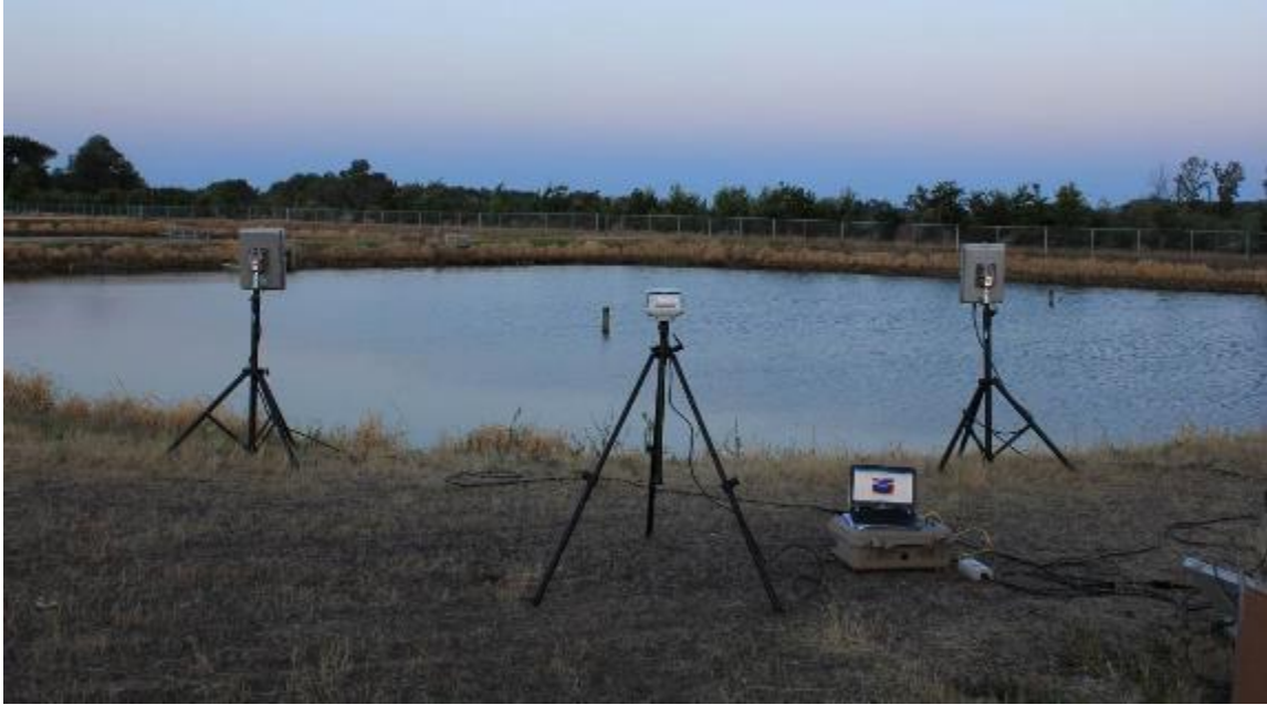
Figure 5. Positioning of the NRG Systems' deterrent near the edge of a pond. A thermal video camera is positioned between two deterrents.
