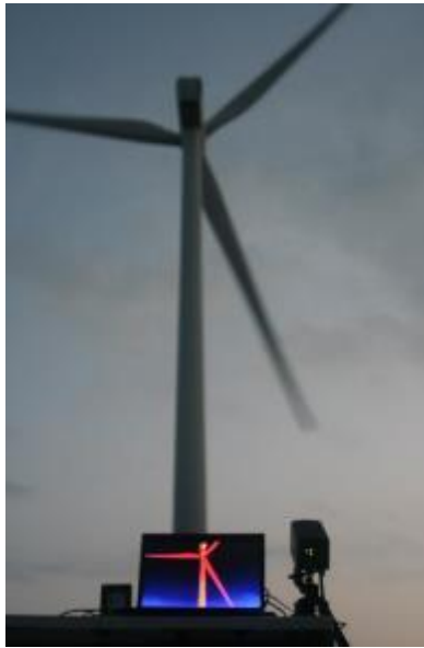
Figure 11. Thermal video camera and laptop positioned near a wind turbine.
