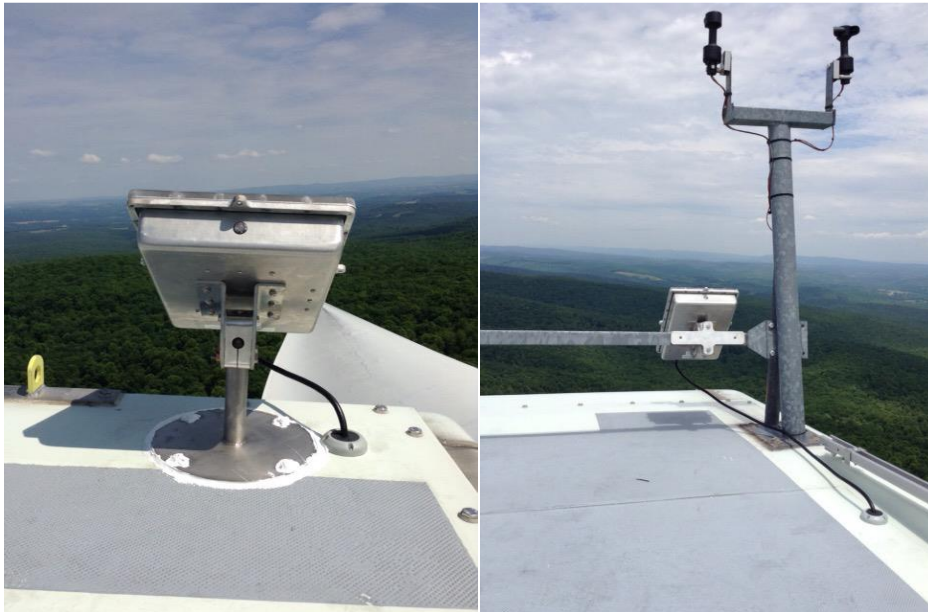
Figure 2. Photographs of an ultrasonic acoustic deterrent mounted near the front of the nacelle pointing perpendicular to the nacelle (left), and an ultrasonic acoustic deterrent mounted near the rear of the nacelle pointed leeward of the nacelle (right).
