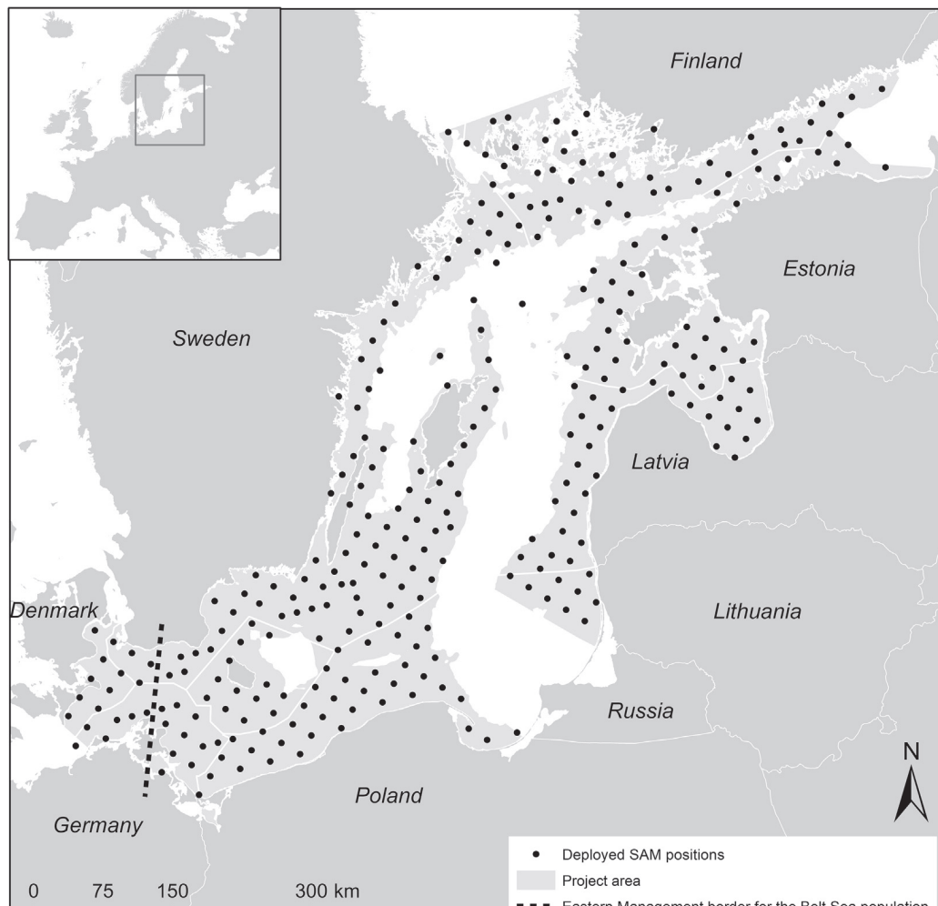
Figure 8. The survey design for the SAMBAH project in the Baltic Sea. The black dots show the 304 acoustic monitoring stations for harbour porpoises placed on a systematic sampling grid (from Carlén et al. , 2018). The study area covered was 166,800km 2 .
