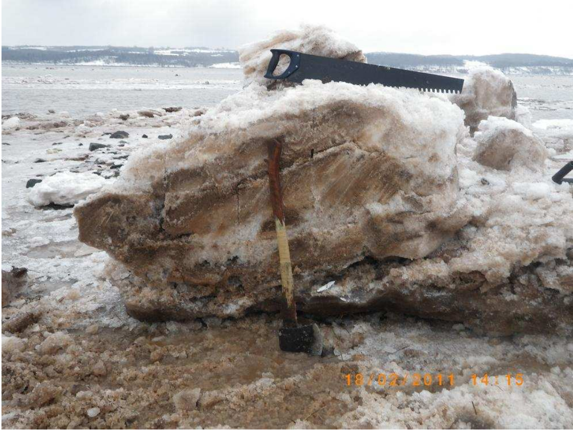
Figure 3: An ice cake has been sectioned. The axe is 83.5 cm long. Samples of ice were cut from each layer in order to measure their density and porosity. This photograph was taken at 14:15 on 18 February 2011 from the beach at Block Wharf Road, Summerville. The background view looks across the ice rafts on the Avon River towards the Hantsport - Blue Beach coastline.
