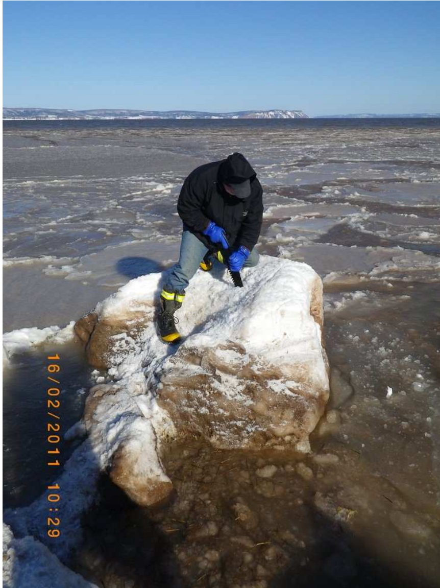
Figure 5: Photograph of ice cake 1 at Evangeline Beach ( 45.13834^{\circ} N, 64.31901^{\circ} W) on 16 February 2011. The tide has yet to recede to the base of the ice cake. A preliminary sectioning cut is being made.
