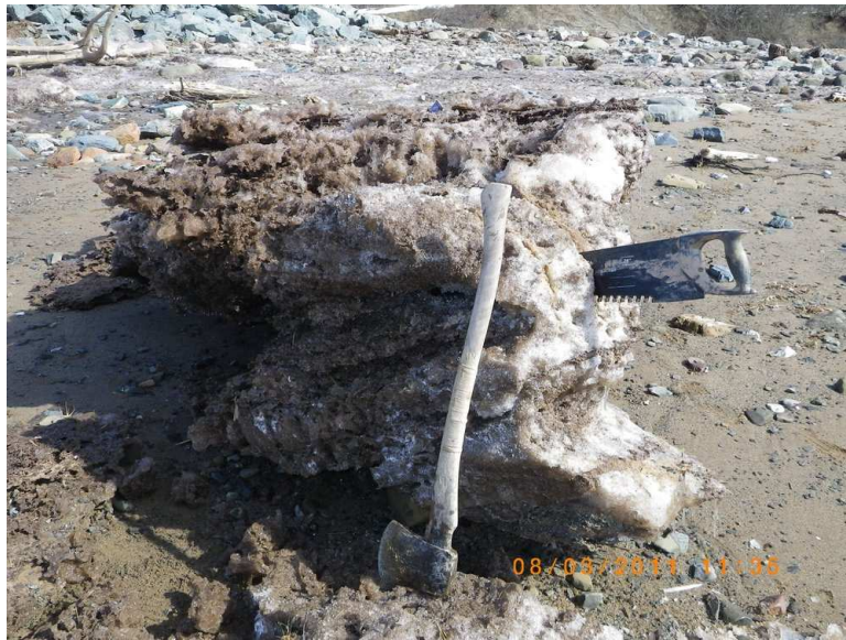
Figure 20: This is ice cake 7 which we sampled for density and porosity measurements. Samples from this ice-block were less dense than the sea water except for one sample from the bottom layer. The GPS location was 45.09785^{\circ} N, 64.18295^{\circ} W.
