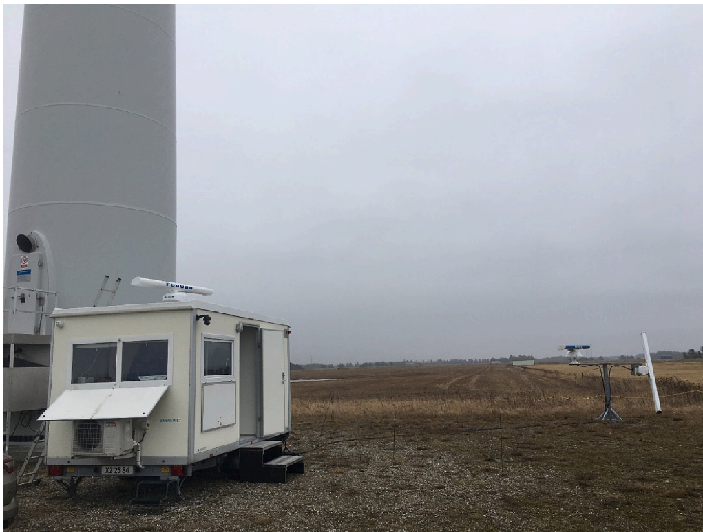
Fig. 4. Image of data collection site at base of turbine #223. On the right are the two Furuno FAR-2127 x-band marine radars (horizontal & vertical); on top of the trailer is the solid-state Furuno DRS25A-NXT radar.
