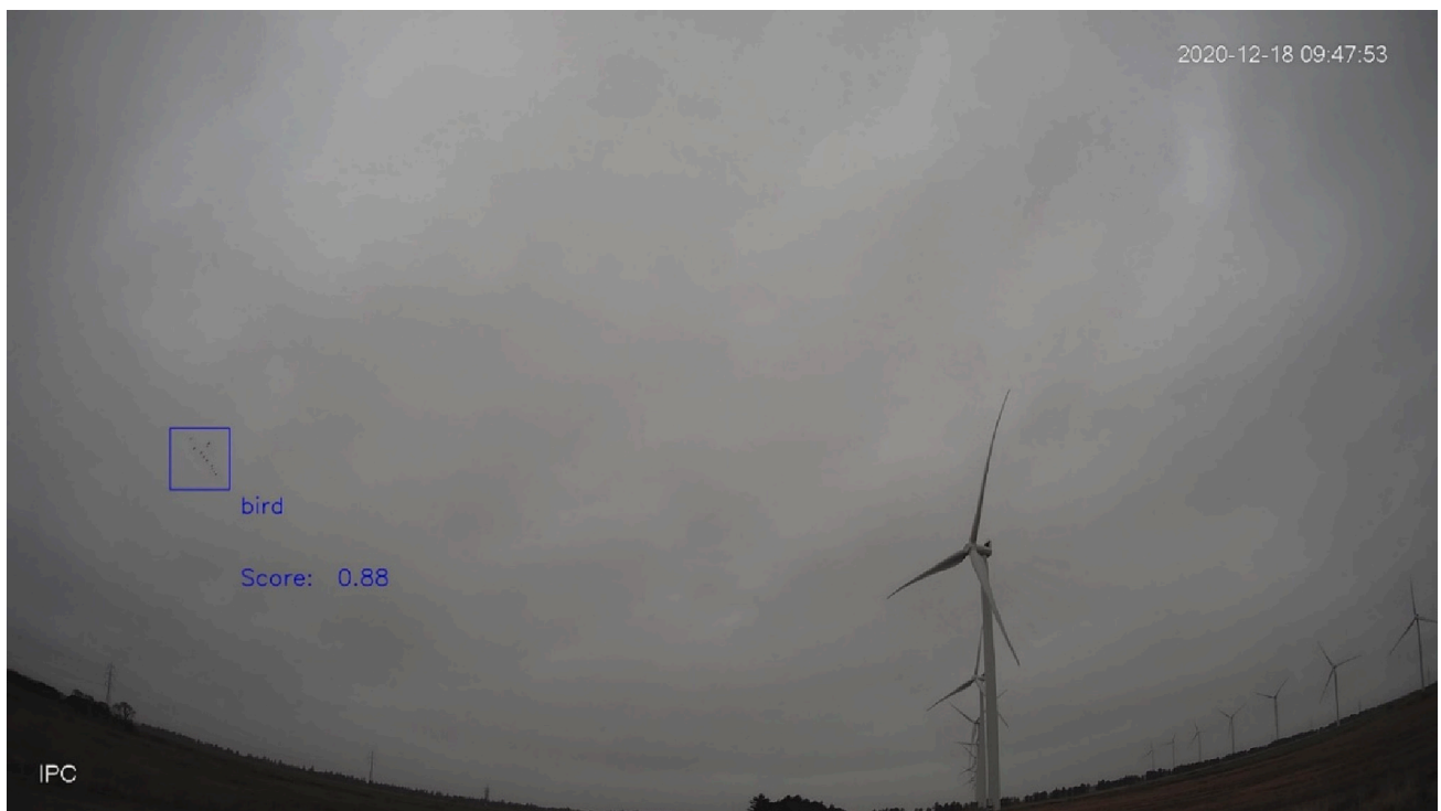
Fig. 8. Prediction score generated by the YOLO model; score of 0.88 on a flock of birds.
