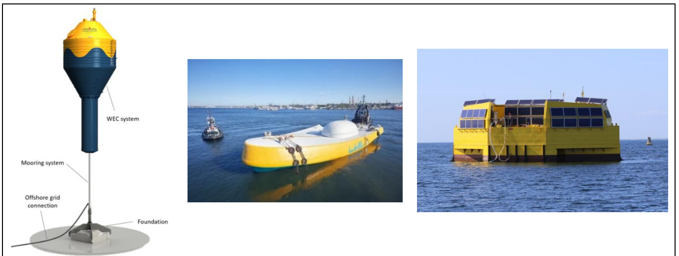
Figure 1. Devices under monitoring of EMF. Left: HiWave-5 (CPO). Centre: Penguin II (Wello). Right: WAVEGEM (GEPS Techno).
