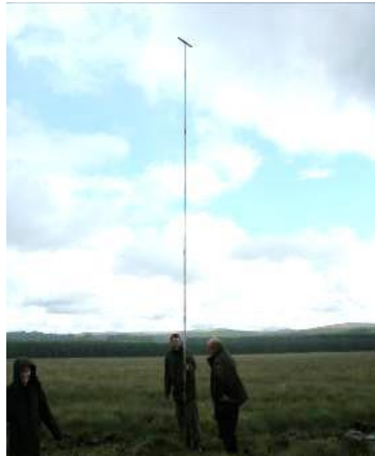
Thorough site investigation, such as detailed peat depth surveys, is essential at the early stages.
