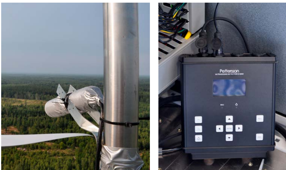
Figure B 4.2 An ultrasonic microphone mounted on the nacelle house and connected with a bat detector inside the tower via a cable.
