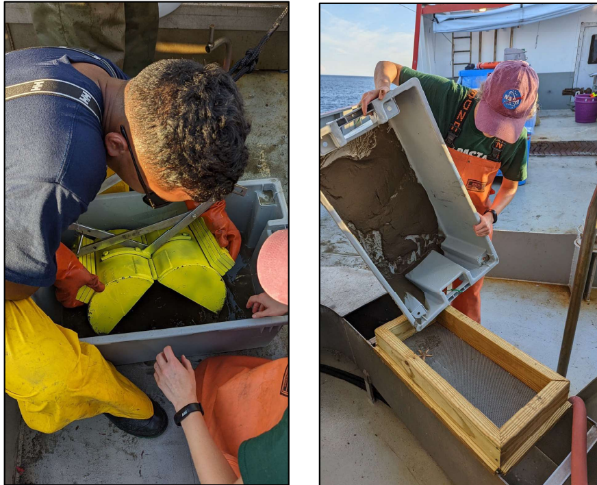
Figure 13. (Left) Peterson grab sample collection. (Right) Benthic sediment sample is collected and placed into a bin. Sample is then sieved through mesh and retained for lab processing.
