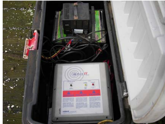
Figure 3-10. Electronic acoustic harassment devices that are used to deter animals (e.g., Pacific harbor seals, California seal lions) from damaging property might also be useful for safely excluding marine mammals, fish, and marine turtles from an ocean energy installation. Source: NOAA
