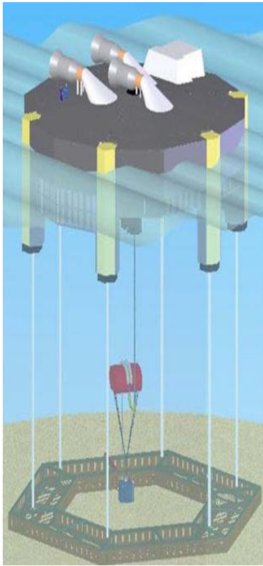
Figure 3-4. The ORECon Multi Resonant Chambers (MRC) device deploys multiple OWCs around a 40-meter platform tethered to the sea floor offshore. Source: ORECon
