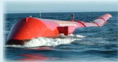
Attenuator (Pelamis) Source: Pelamis Wave Power
