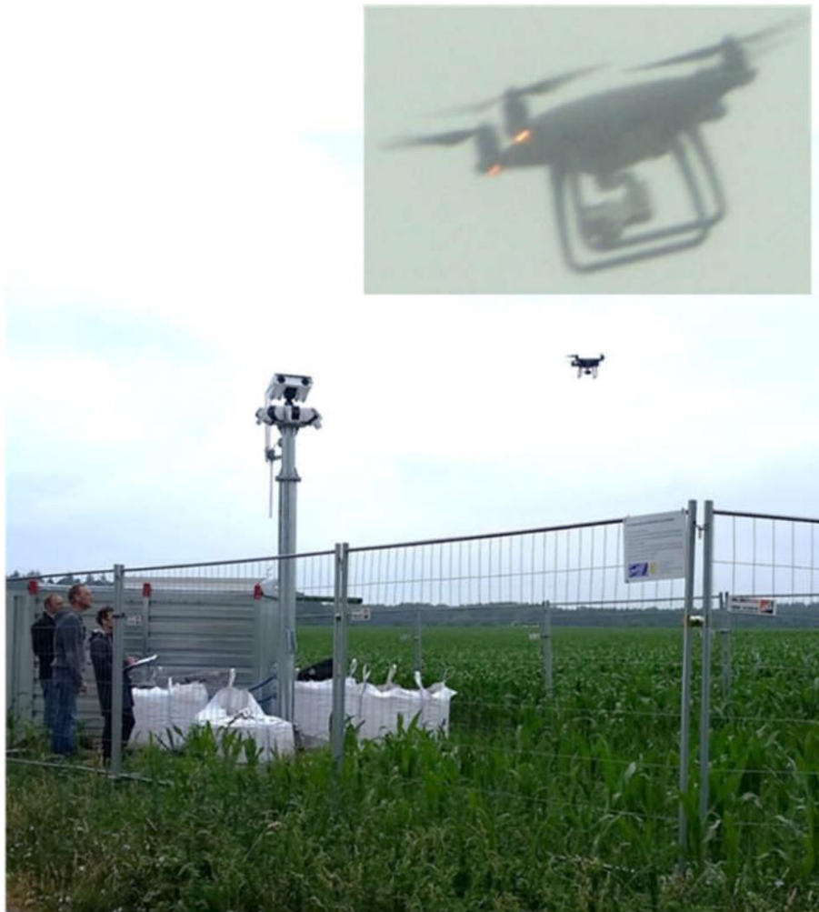
Figure 26: Acquisition test with a GPS-located drone. The small picture shows a picture of the drone by the IDF from a distance of approx. 150 m.
