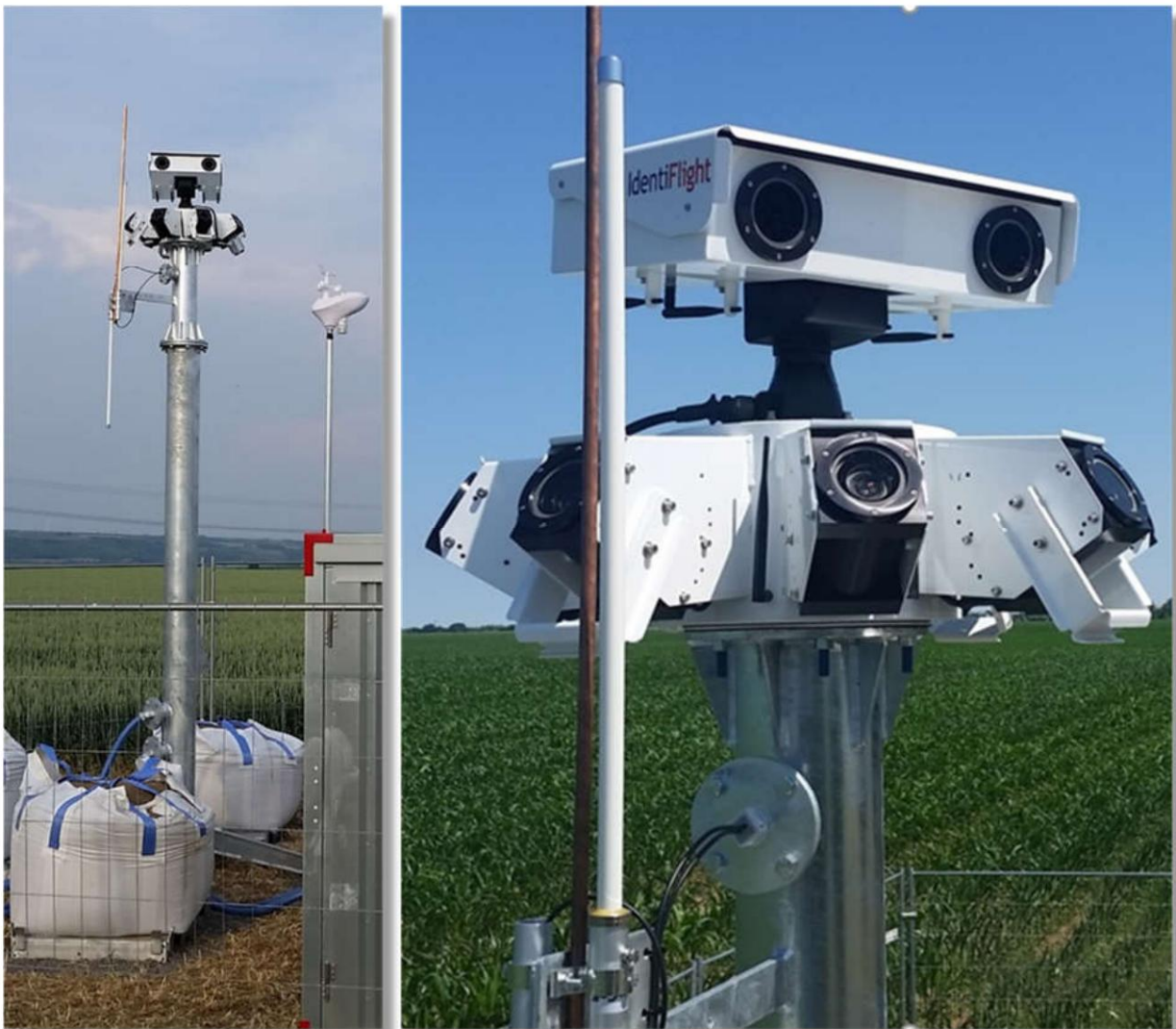
Figure 2: The IdentiFlight system, consisting of 8 wide-angle cameras and a movable one Stereo camera.
