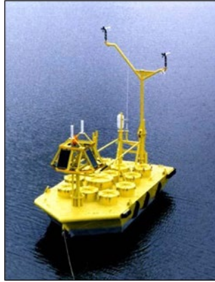
Figure 5: 6-Meter Boat-Shaped Hull Buoy Source: NDBC (2012)
