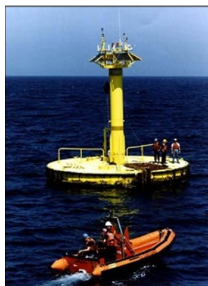
Figure 4: 10-Meter Discus-Shaped Hull Buoy Source: NDBC (2012)
