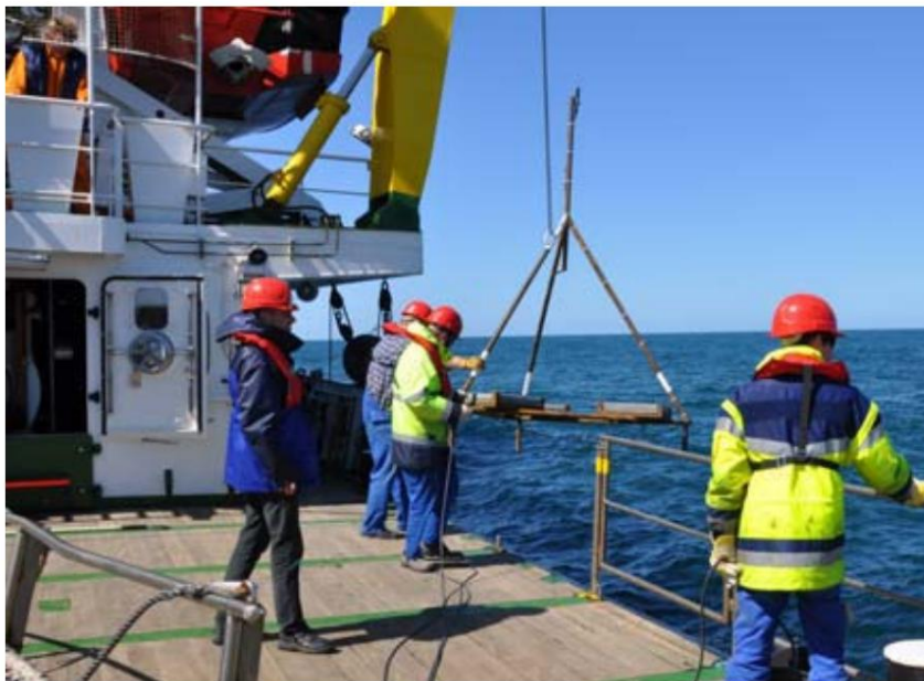
Fig. 6.1.1: Deposition of the hydrophone at the AV04 system (Photo: BSH)
