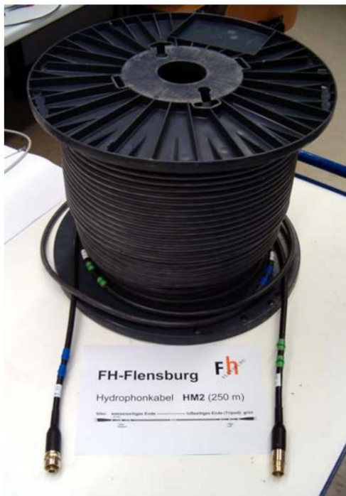
Fig. 5.2.5: Hydrophone cable, ready-made
