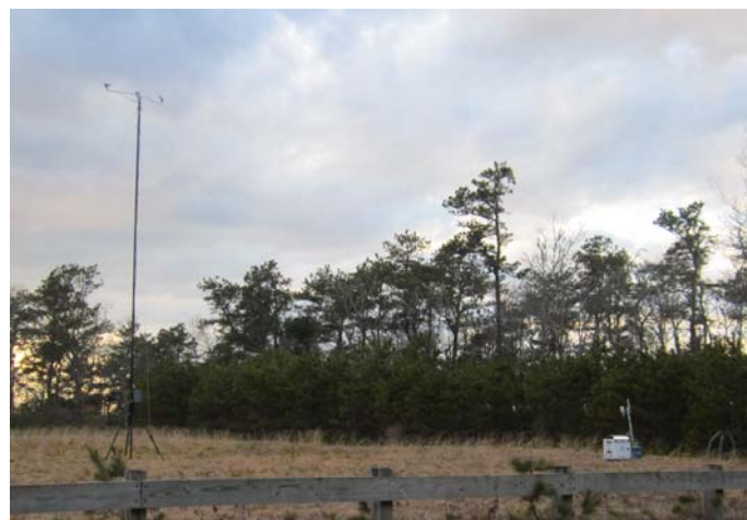
FIGURE 86: 10-METER MET MAST ON LEFT WITH LIDAR ON RIGHT
