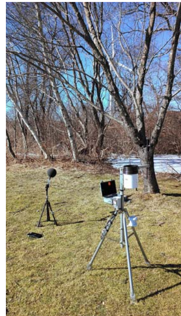
FIGURE 85: SOUND LEVEL METER IN BACKGROUND AND GROUND MET EQUIPMENT IN FOREGROUND
