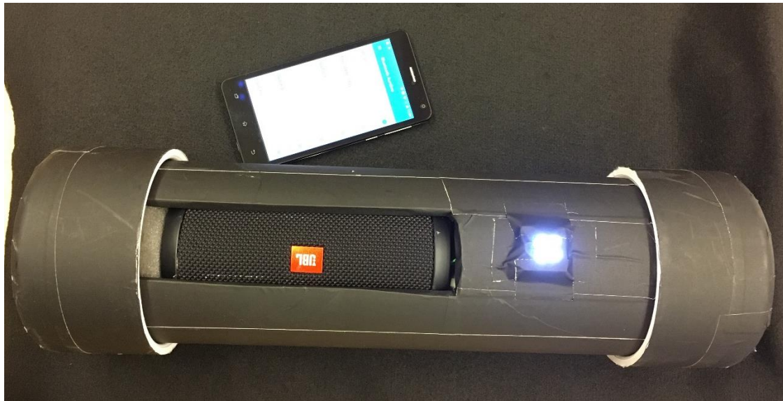
Figure M2. Refined stimuli playback system used for the second round of behavioral tests with Golden and Bald Eagles. LED light panel is seen with the white LEDs in place and turned on.
