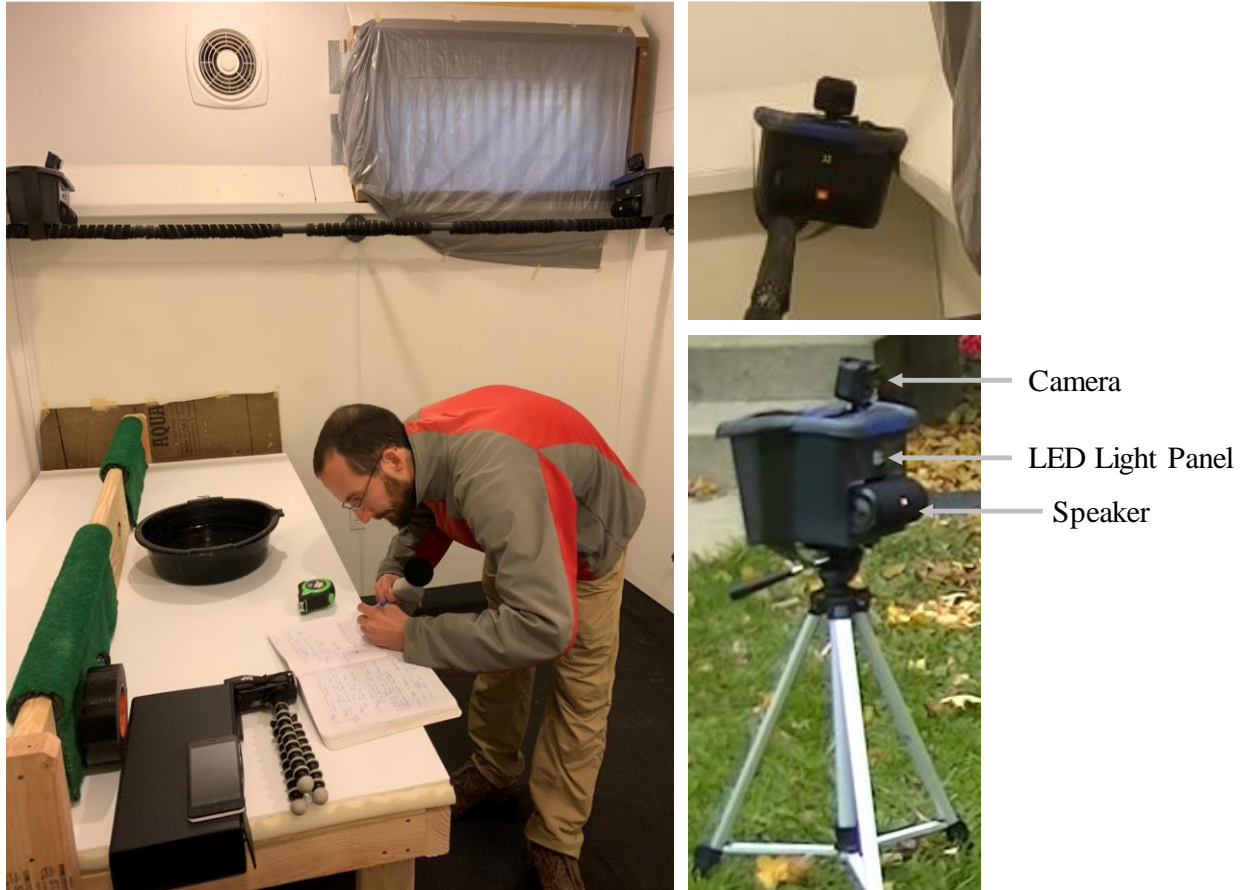
Figure M1. Stimuli playback system prototype in initial housing. This model was tested with a Red-tailed hawk falconry bird and is seen here within the hawk's indoor enclosure and when deployed outdoors.
