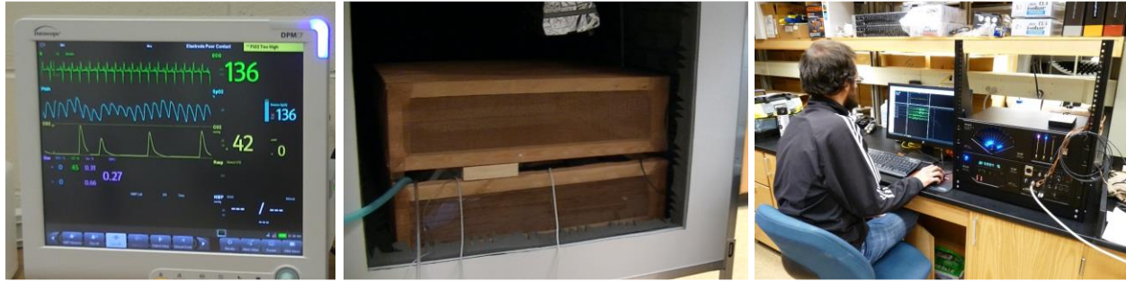
Figure F1. Testing the anesthesia protocol, anechoic chamber, and TDT on the Canada Goose. Panels show the vitals being monitored (a) on the goose under anesthesia in the anechoic chamber (b) and the resulting data collected on the TDT (c).
