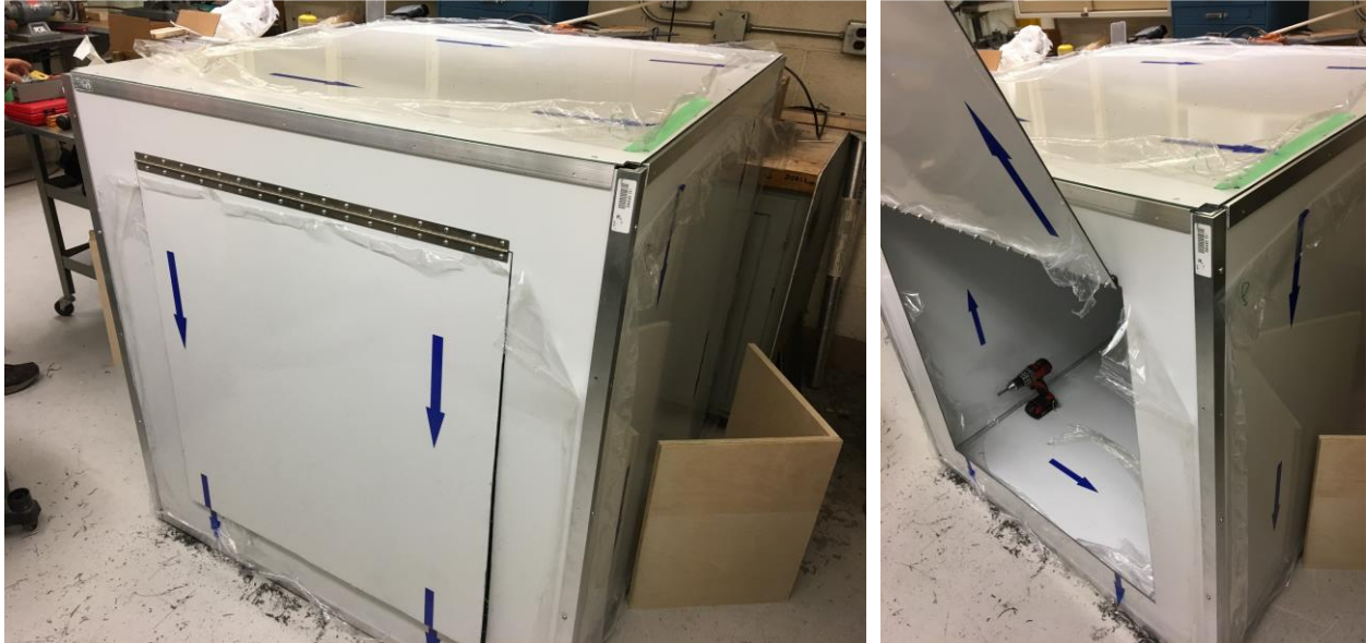
Figure C1. Portable anechoic chamber structure after completion of the build and before application of the acoustic foam panels.
