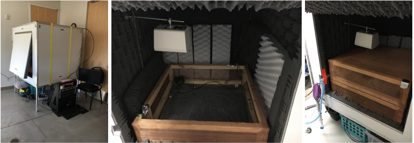
Figure C2. Portable anechoic chamber complete with installed foam panels installed, Faraday cage, and testing equipment ready for measurements at a rehabilitation center.
