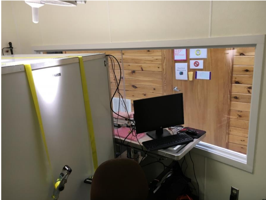
Figure I3. The anechoic chamber was placed in a location determined by the wildlife or rehabilitation center. Electronics for generating stimuli and recording auditory responses from eagles were outside the anechoic chamber.
