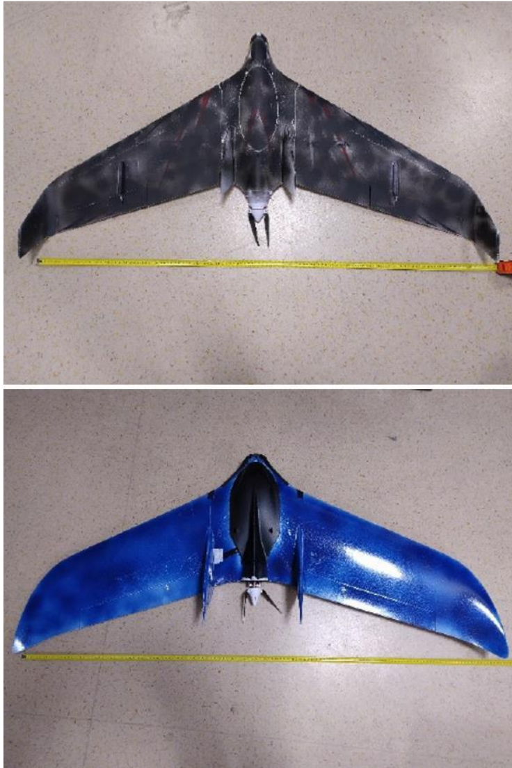
Fig. 2.9: Drones used for position accuracy determination, wingspan of 1.5 m and 2 m (photo: PNE 2023).
