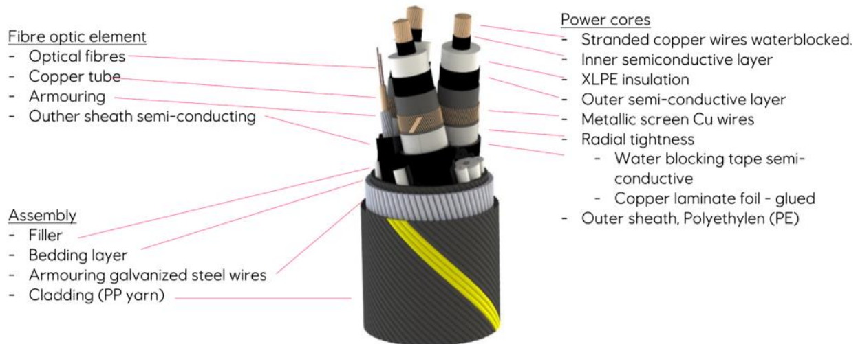
Figure 3.3-9 Representative Interarray Cable
