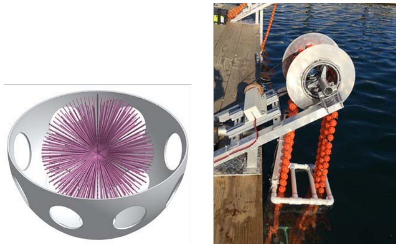
Figure 6.6. Adsorbent material encapsulating a protective sphere (left), and symbiotic machine for ocean uranium extraction (right). Source: Haji et al. (2017a)
