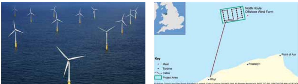
Figure 1: Showing an aerial photograph (left, reproduced courtesy of Anthony Upton (info@anthonyupton.com)) and the site plan of North Hoyle offshore wind farm (right, reproduced courtesy NPower Renewables) located 7km from the N coast of Wales between Rhyl and Prestatyn. The site plan illustrates the five rows of 6 turbine towers (30 in total) and two meteorological masts in around 12m of water.
