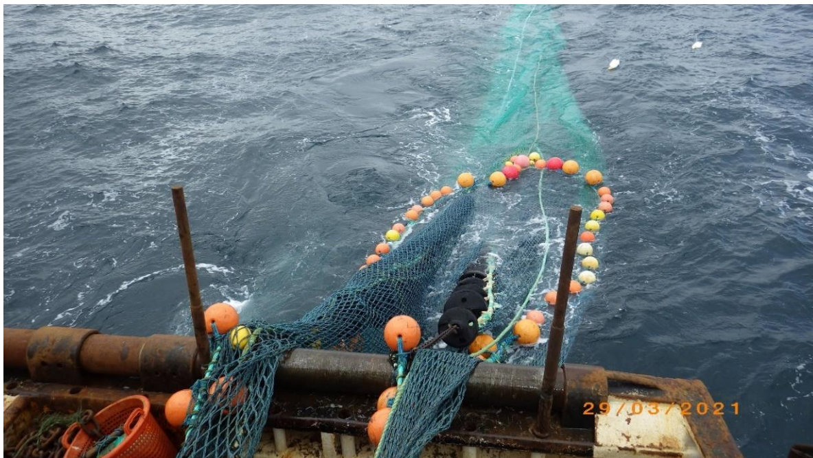
Figure 3.2 Rock-hopper otter trawl used
