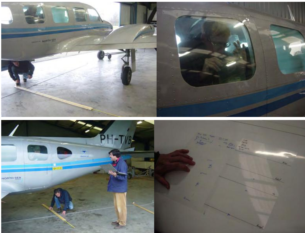
Calibration of observer and side specific strips for the two-engine survey aeroplane PH-TVB during an annual ground truthing session. In the upper right picture an observer is determining his strip by drawing his inner, middle and outer line of his strip. Based on goniometric calculations the strip can be determined and compared with the goniometric calculations of the strip measured on the floor of the hangar.
