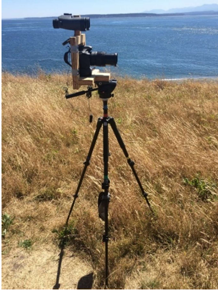
Figure 7. Vantage-point equipment setup. Canon DSLR camera capable of both still image and video footage mounted with compass-reticule binoculars in a custom-built frame. The tripod legs were marked to ensure that the system was set up in the correct position at the start of each day above our surveyor's mark and the height measured to ensure that the camera was always at the same height. A specialized video tripod mount allowed for smooth panning across the survey area.
