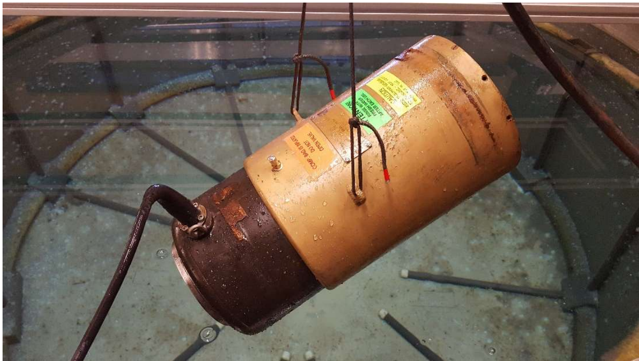
Figure 2. J11 sound transducer after testing in a lab tank.
