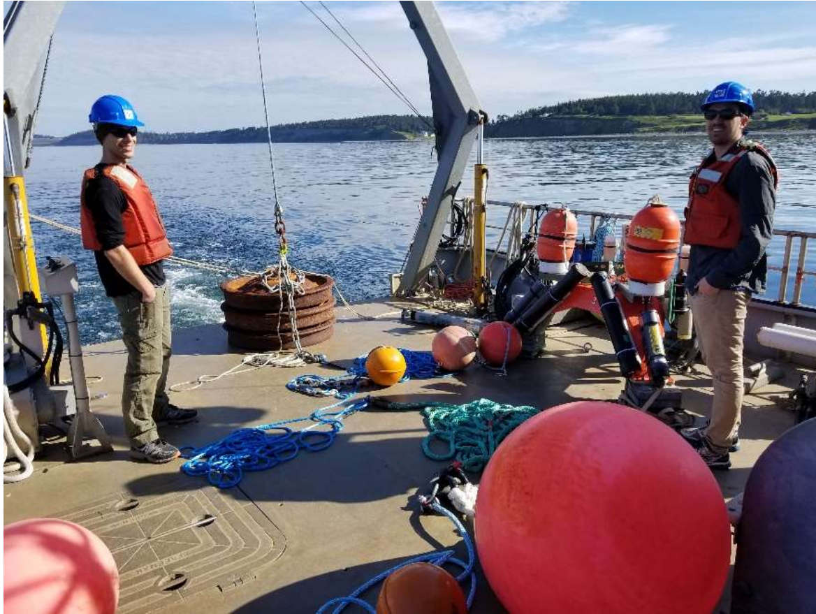
Figure 5. Mooring wheel stack and Sea Spider aboard R/V Jack Robertson prior to deployment
