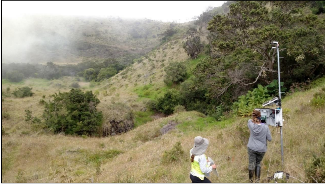
Appendix I Figure 3. Pu'u Makua bat acoustic recording site AUW4. The two microphone models (SMX-US and SMX-U1) are shown attached to the top of the pole, demonstrating comparison testing set up.
