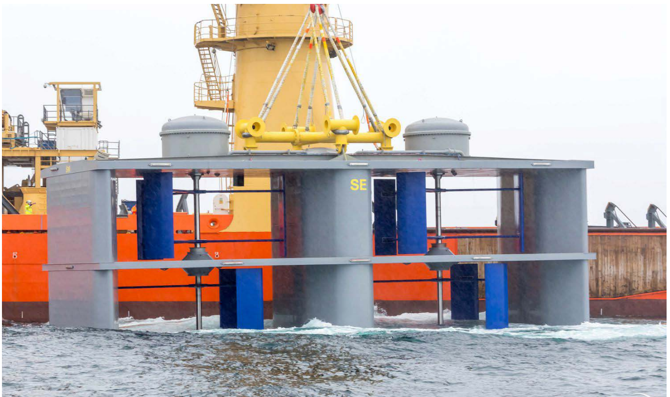
Figure 16. 1MW turbine deployed on Paimpol-Bréhat test site in Brittany (source: HydroQuest).
