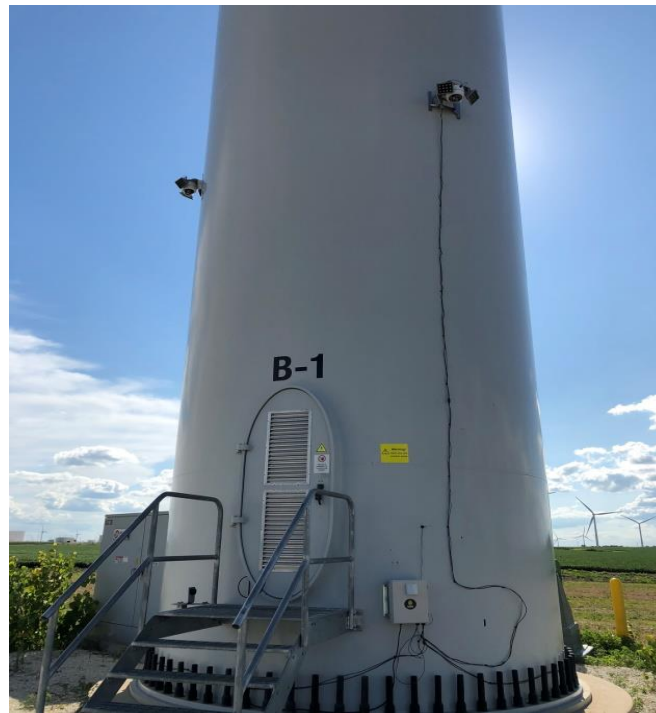
Figure 3. A photograph showing NRG Systems' Bat and Avian Mortality Monitoring System. The cameras were mounted approximately 7.6 meters (25.0 feet) above the ground and pointed downward.
