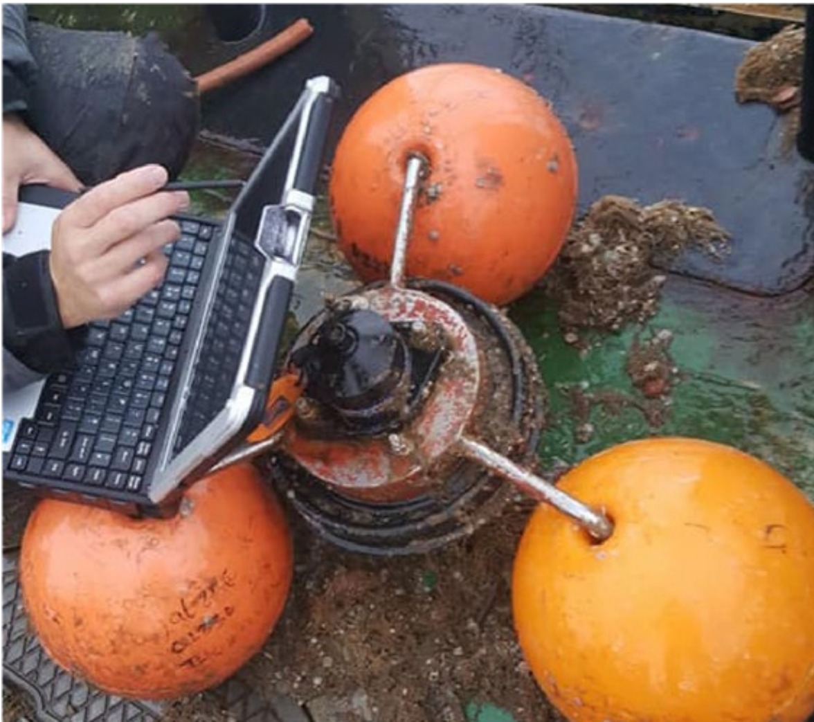
Figure 50: Downloading data from the acoustic receiver. Photo credit: Andy Holbrow, Atlantic Diving Services Ltd.
