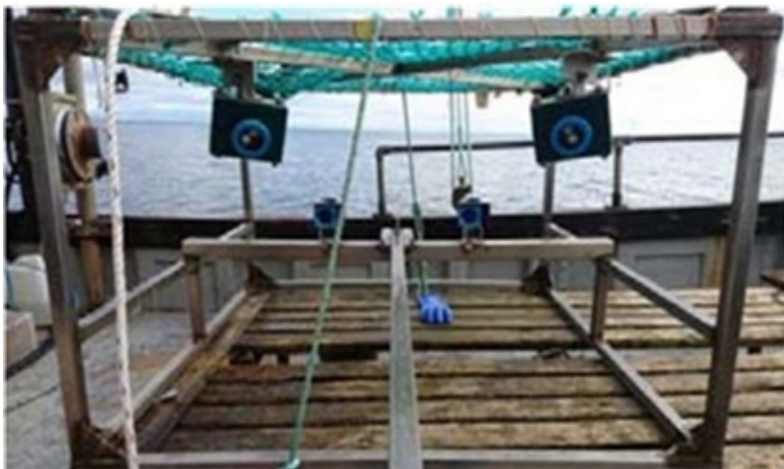
Figure 43: Stereo Baited Remote Underwater Video Camera (SBRUV) frame.
