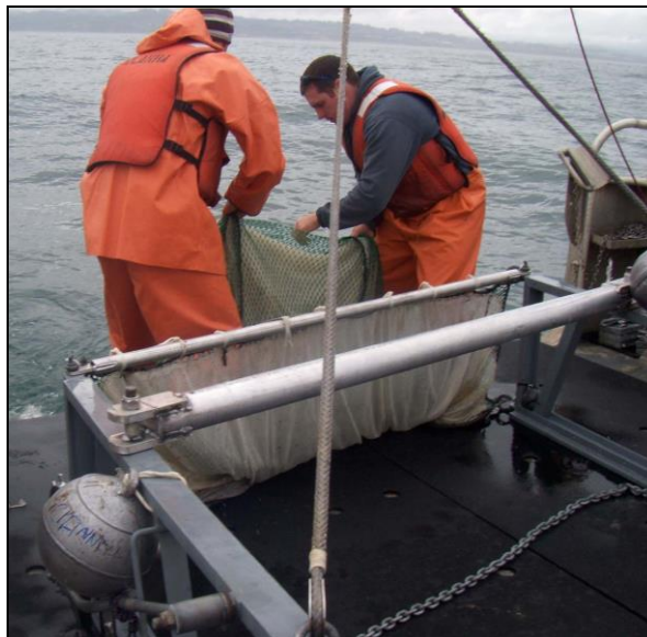
Figure A1: Beam trawl used for capturing juvenile groundfish and epibenthic invertebrates.
