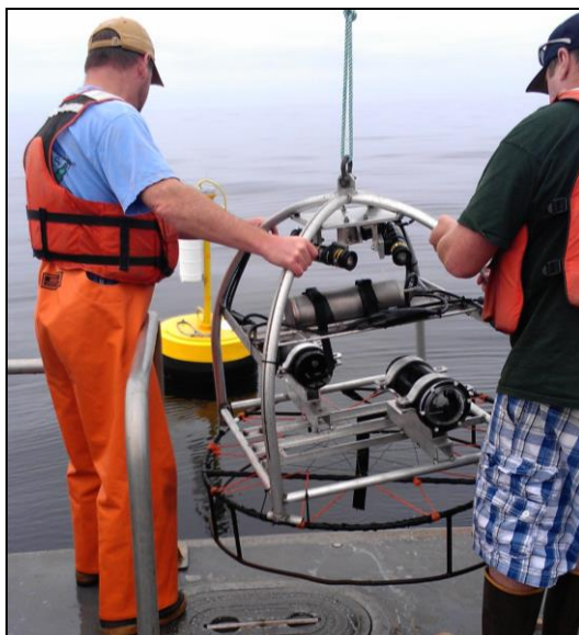
Figure A2: Video lander ready to be dropped near the Ocean Sentinel anchor.
