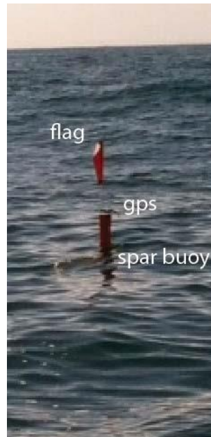
Figure B2: A photograph of the autonomous drifting underwater hydrophone (ADUH) buoy system deployed for acoustic recordings near the Ocean Sentinel at the NETS on September 26, 2013.
