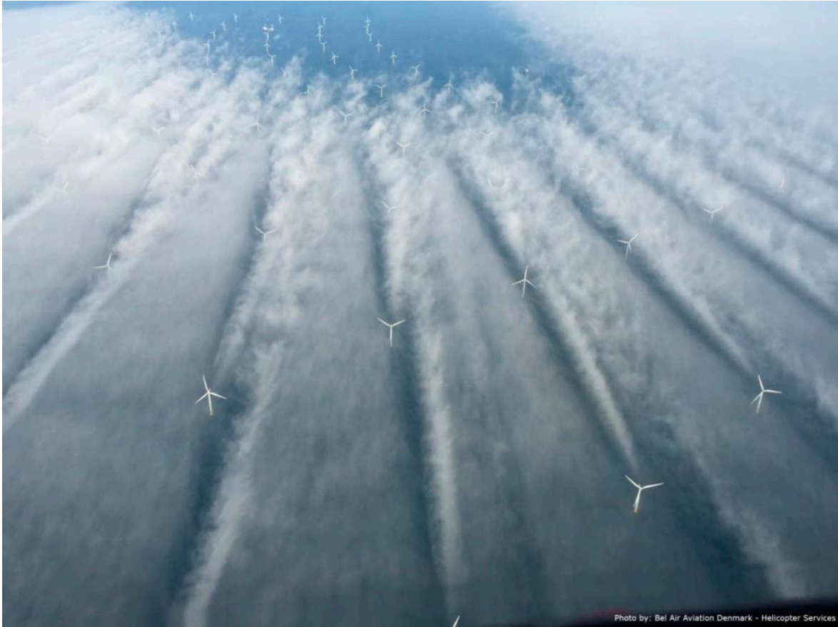
Figure 5.6 Exemplary photograph of the wind-wake effect at Horns Rev II after (HASAGER, 2017)
