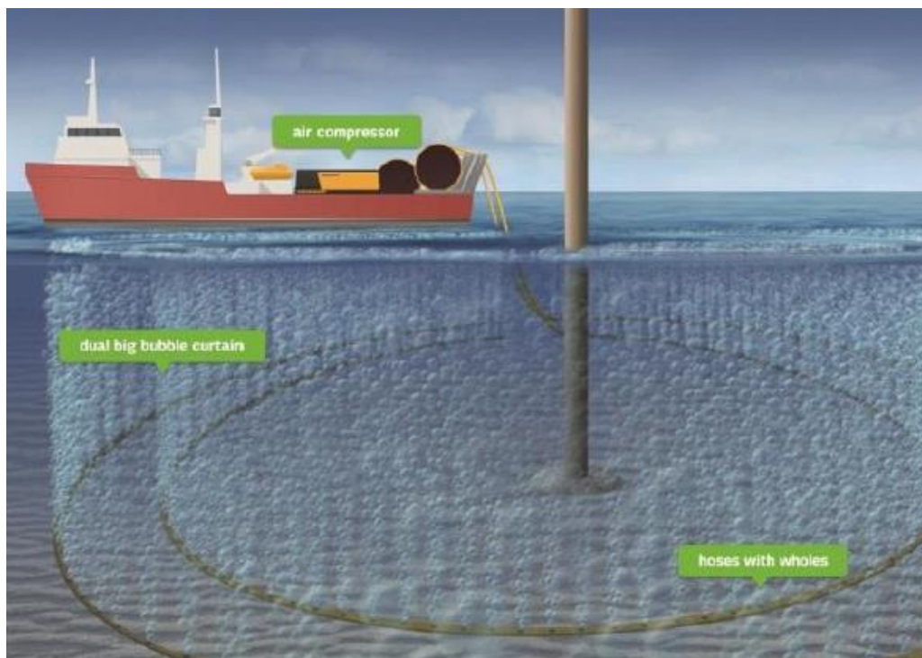
Figure 6.8 Schematic of a double 'big bubble curtain' (RUMES et al. 2016)
