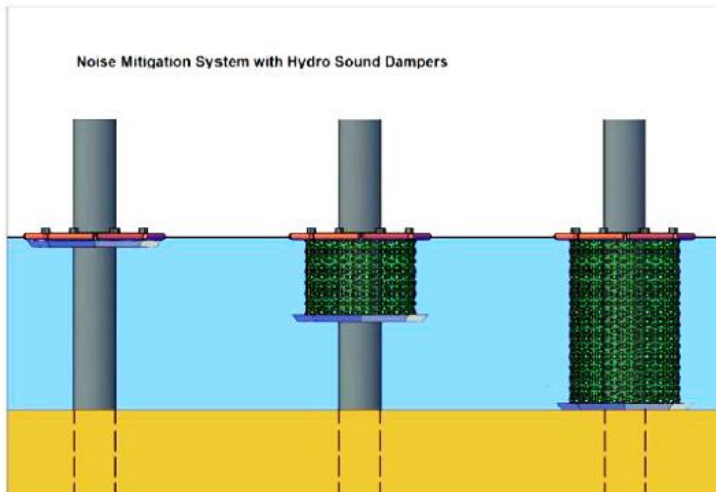
Figure 6.10 Schematic of the HSD single-net system (KOSCHINSKI & LÜDEMANN 2013)
