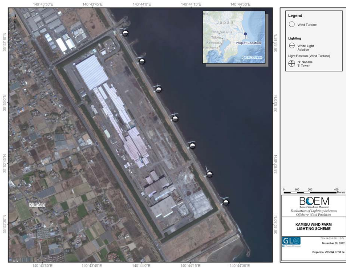
Figure 7-2: Kamisu Wind Farm lighting scheme
