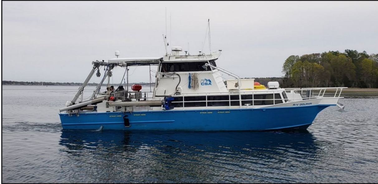
Figure 2. The 49 ft (15 m) R/V Dolphin utilized during the Block Island Wind Farm Geophysical Survey with starboard side pole mount
