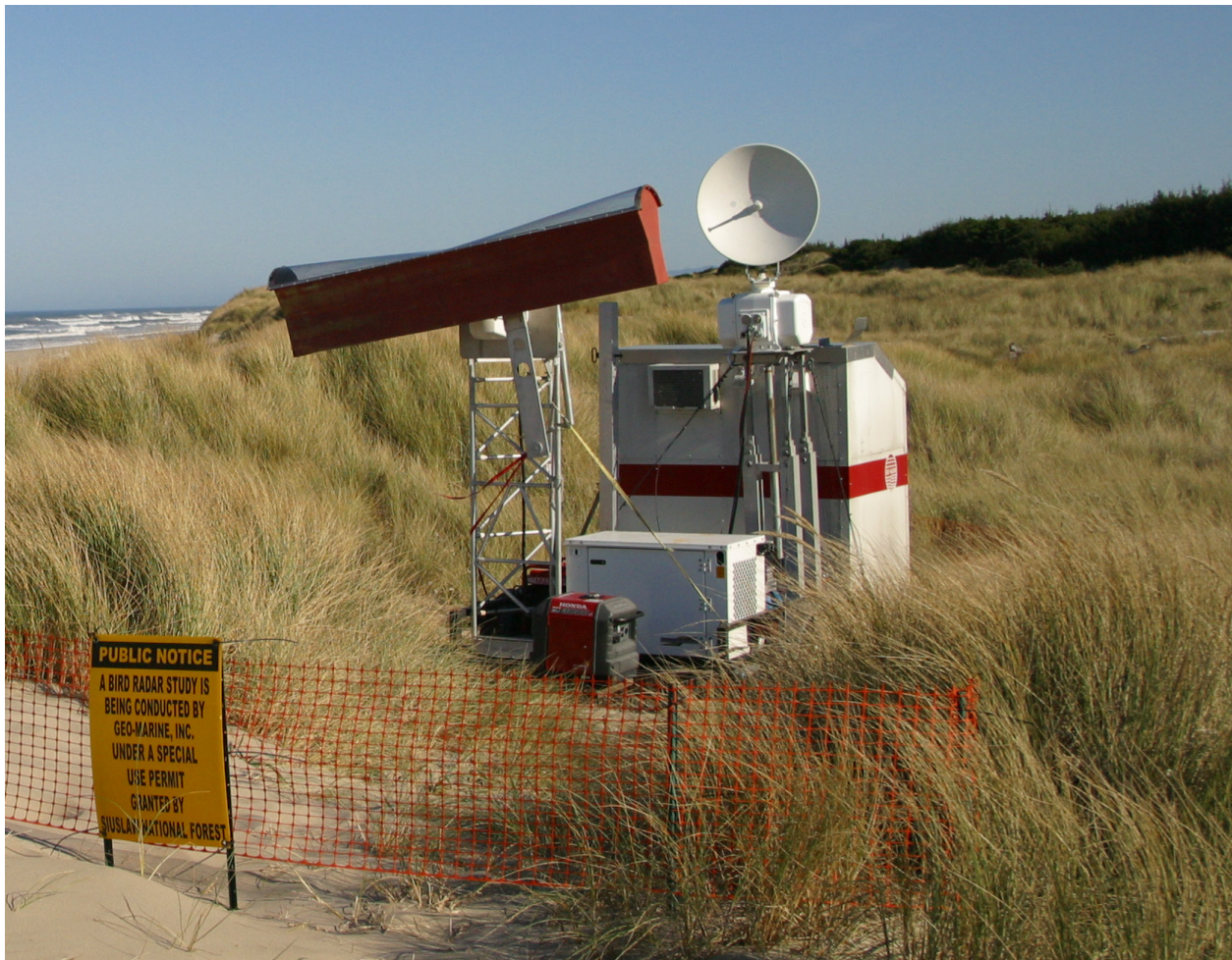
Figure 4-1. GMI MARS ® System showing both VerCat (vertically scanning) antenna (left) and TracScan (horizontally scanning) parabolic dish antenna (right) and transmitter/receiver unit.
