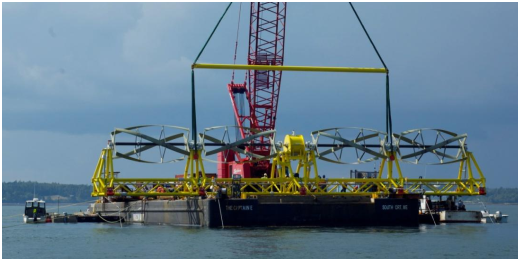
Figure 3. TidGen® Power System, deployed in 2012-2013 in Cobscook Bay, Maine
