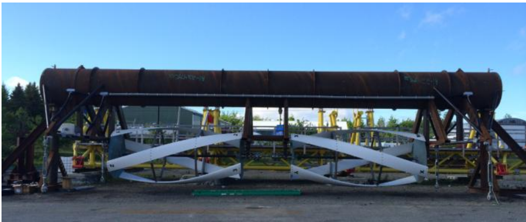
Figure 4. OCGen® module, deployed in 2014, Cobscook Bay, Maine
