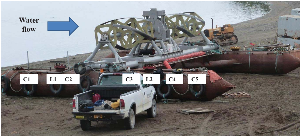
Photo 1. ORPC device before deployment, showing approximate mount locations of underwater cameras (C1 – C5) and lights (L1 – L2) in 2014. Water would flow from left to right.
