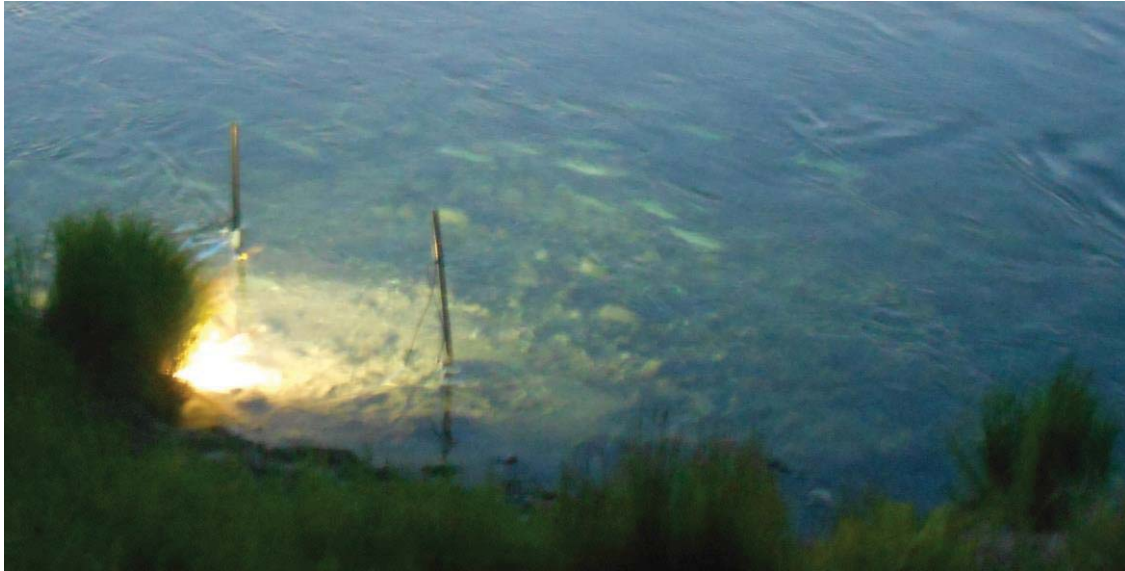
Photo 5. Surface view of pre-deployment testing of the underwater lights at 1:00 AM on July 3, 2014. Approximately ten sockeye salmon are seen migrating within the illumination field, at the top center of photo. Image is from a conventional (not underwater) camera, from about 20 m away.
