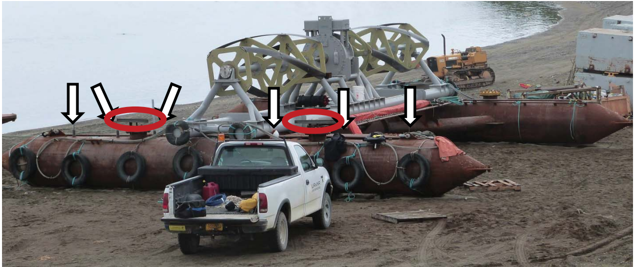
Figure 2. Location of mounts for six cameras (white arrows) and two lights (red ovals) on the ORPC device. Water would flow from left to right.
