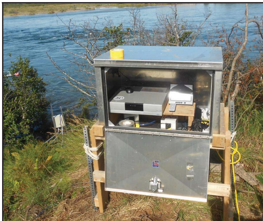
Photo 6. Shoreside cabinetry that housed the video recording system and power link for the BRI RISEC device in 2014. Marker buoys for the submerged device can be seen at top left of photo.
