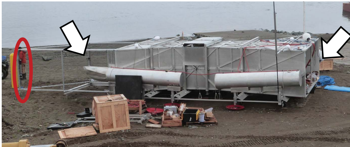
Figure 1. Location of mounts for two cameras (white arrows) and one light (red oval) on the BRI device. Water would flow from left to right.
