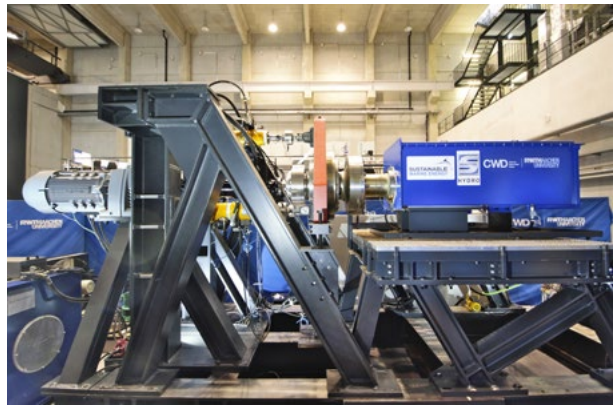
Drivetrain test rig at Center of Wind Power Drives, RWTH Aachen University
