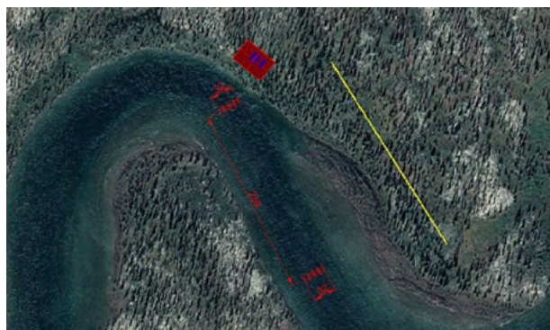
Preliminary site layout with 2 rows of 4 turbines (rated at 50kW with a flow velocity of 3m/s)
