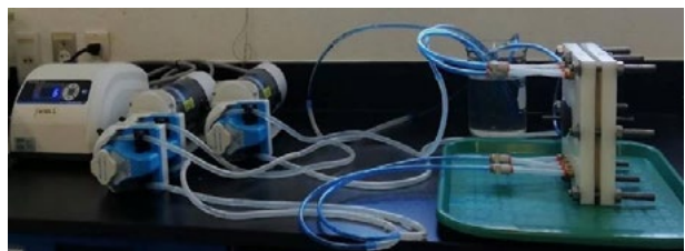
One of the RED salinity gradient energy laboratory prototypes developed by CEMIE-Océano
