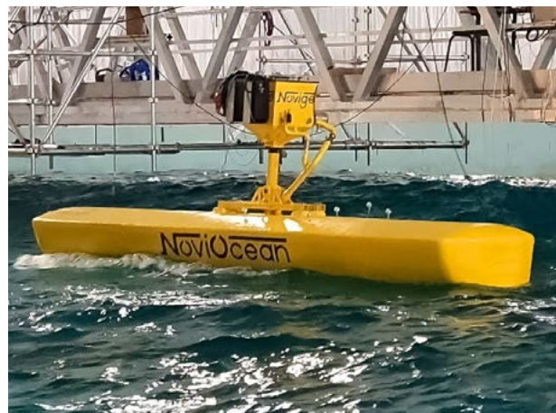
NoviOcean in a towing tank at the Research Laboratory in Hydrodynamics, Energetics and Atmospheric Environment (LHEEA) in Centrale Nantes. (© Novige)
