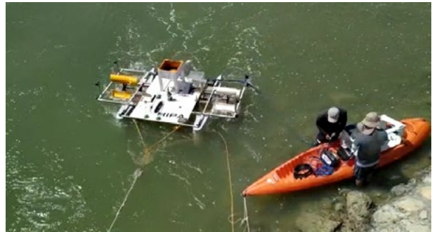
HIPA hydrogenerator testing in the field
