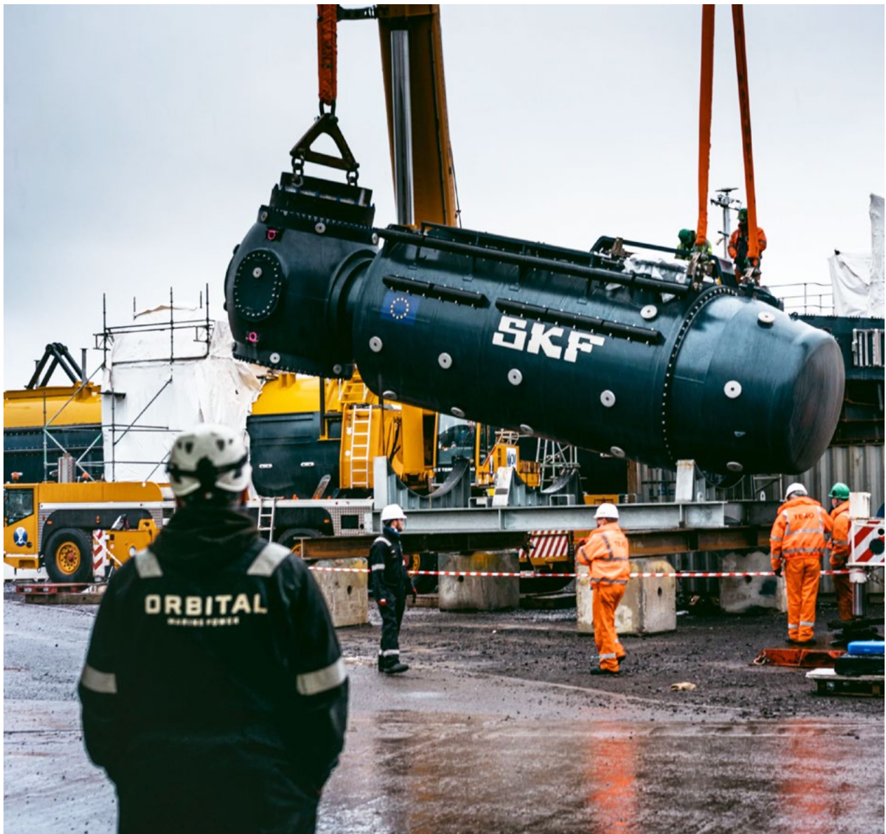
Power train for Orbital Marine Power's O2-2000, developed and manufactured by SKF
