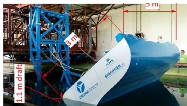
Wave tank experimental test on large scale model of Pivot
