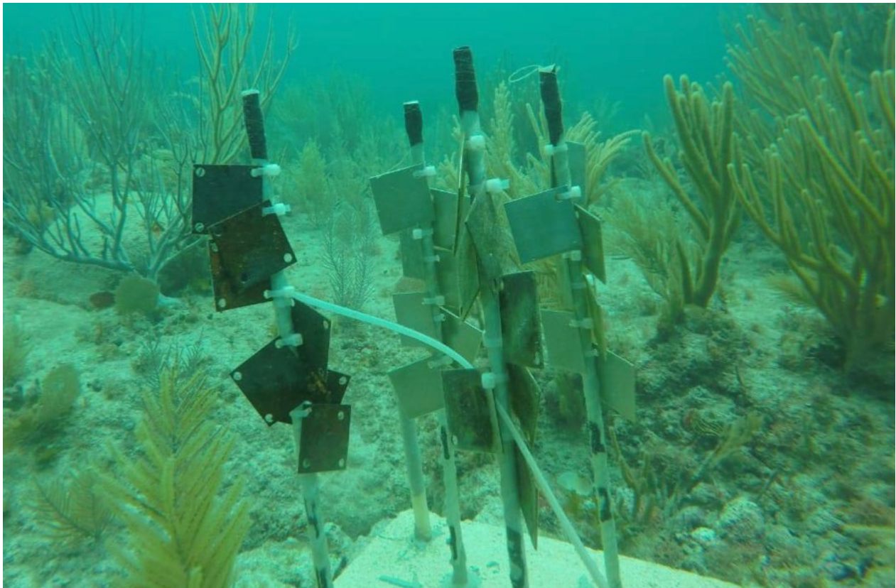
Nanostructured and superhydrophobic materials tests in the Mexican Caribbean
