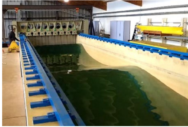
Wave maker at IFREMER Brest wave Canal © Ifremer
