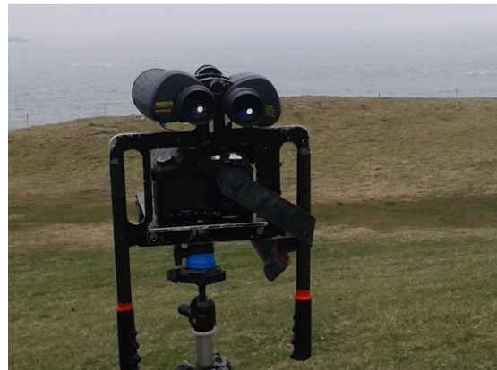
Figure 3. Binocular and camera mount used by SMRU Marine at Skerries.
