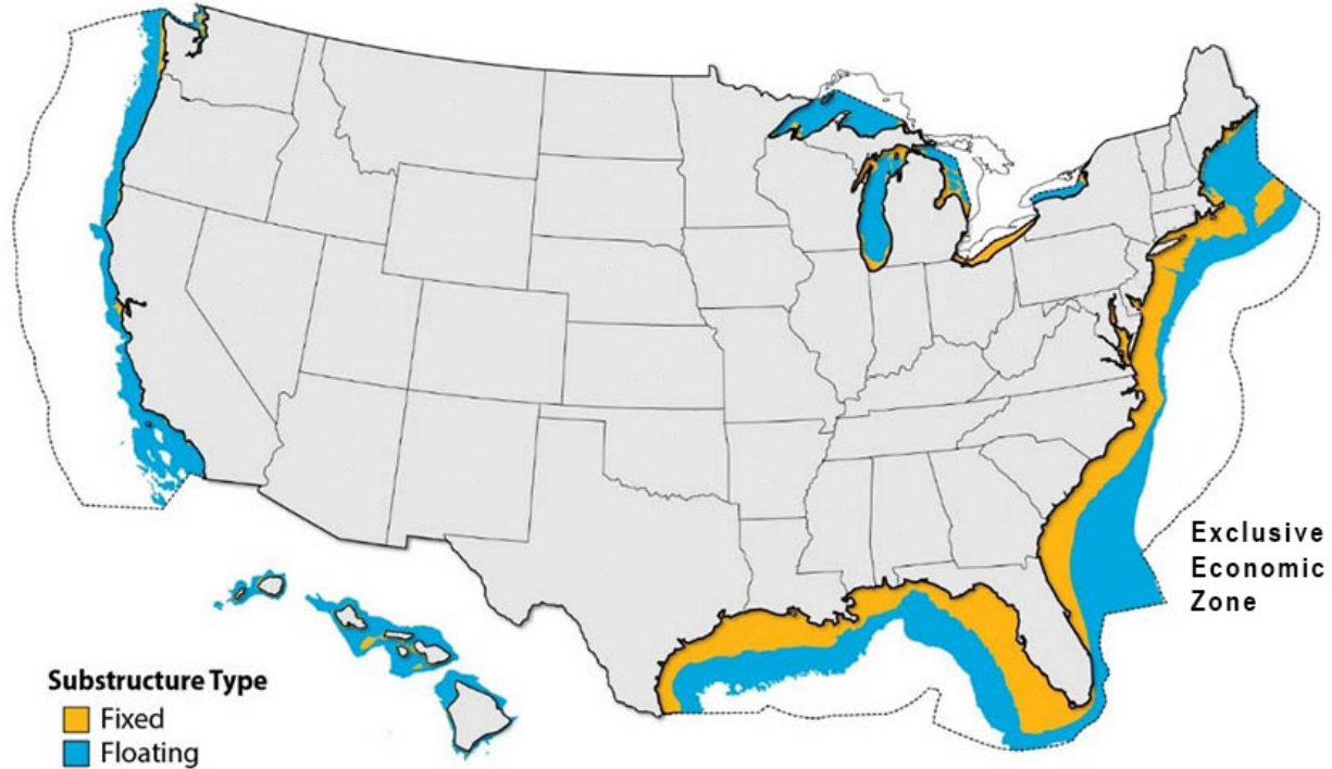
Figure 2. General locations off the coast and within lakes of the United States where water depth (maximum 1300 m [4265 ft.]) and wind speeds are sufficient for installation of fixed-bottom (yellow) and floating (blue) wind energy turbines. Image does not consider potential siting constraints. Modified from a graphic by Philipp Beiter, National Renewable Energy Laboratory.
