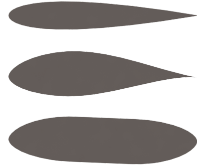
FIGURE 6: HYDROFOIL SECTIONS. FROM TOP TO BOTTOM: NACA 0015; NACA 63-424; BIDIRECTIONAL FOIL.
