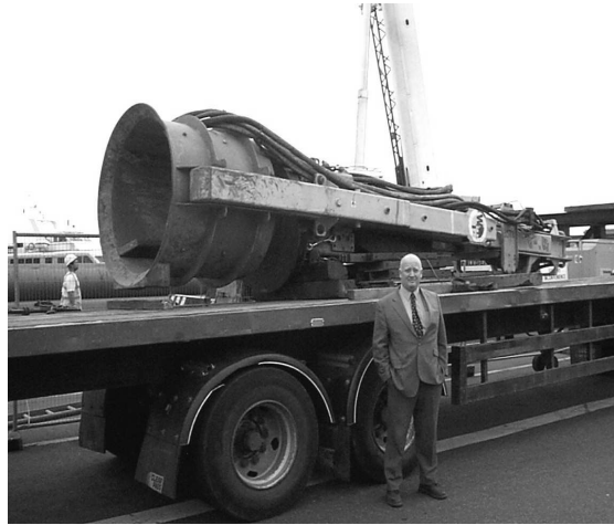
(a). A view of the lower end of the impact driver, while it was lying on a lorry.
