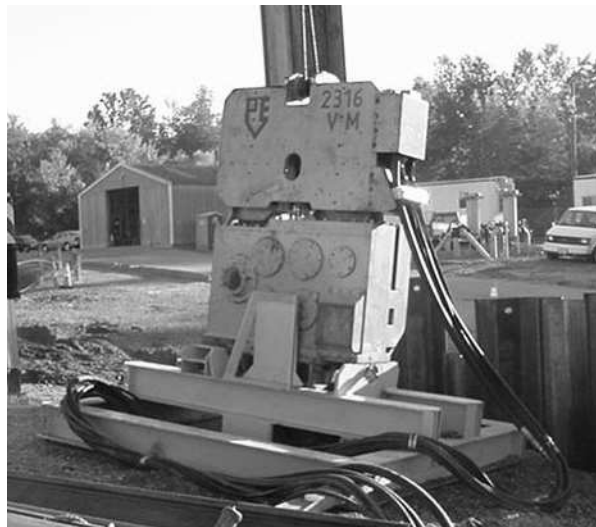
Fig. 10. A PVE 2316 VM vibropiling driver. It is shown resting in a cradle made of I-section beams.
