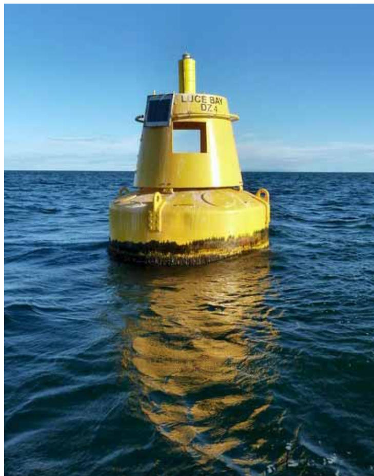
Figure 14.1 Typical yellow special marker buoy
