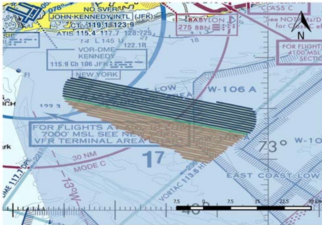
Figure 4. Flight plan used for the Wind Energy Area using image captures for grid survey.
