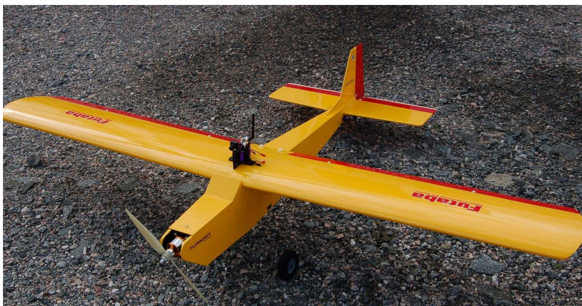
Figure 52. Model aircraft with video camera and transmitter used for radar-performance testing. Photo: Pål Kvaløy.
