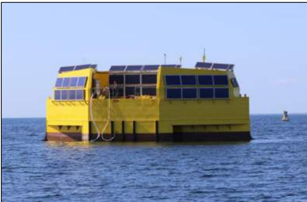
Figure 10. GEPS Techno WAVEGEM (Source: GEPS Techno).
