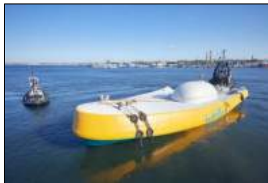
Figure 6. Wello Penguin II WEC (Source: Wello).
