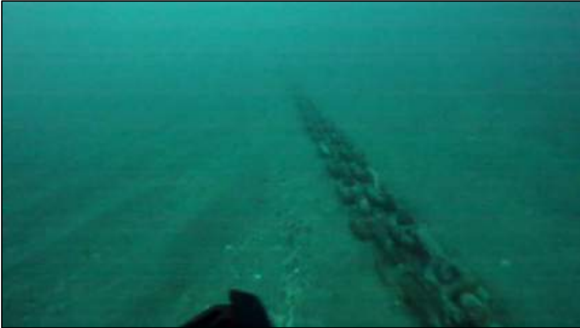
Figure 31. The lower catenary of the mooring leg 1, lying on the bottom.
