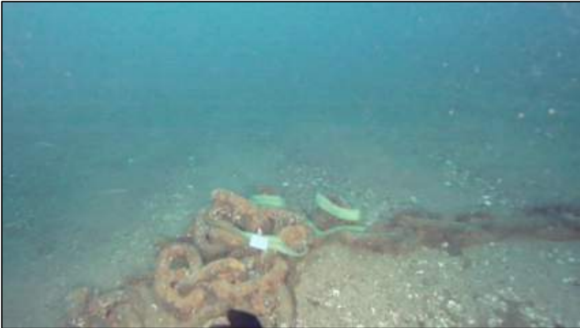
Figure 34. A girth attached to the upper end of the lower catenary of the mooring leg 2.
