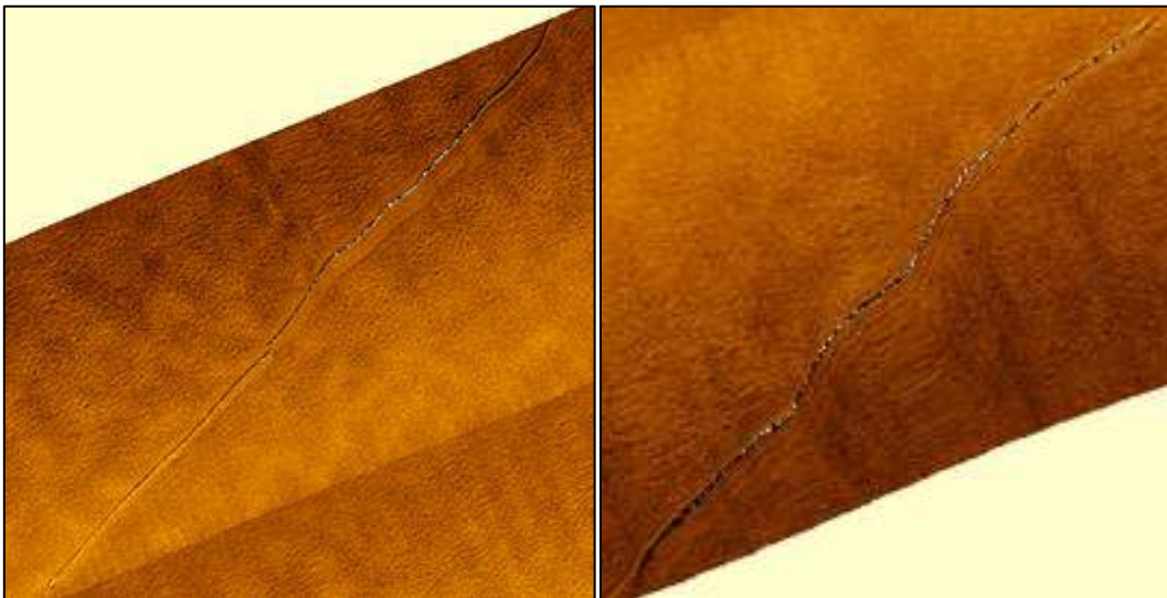
Figure 57. Zoom on footprint - SSS data of mooring line #2 (SW on the left) and mooring line #4 (NE on the right) (09/06/21).
