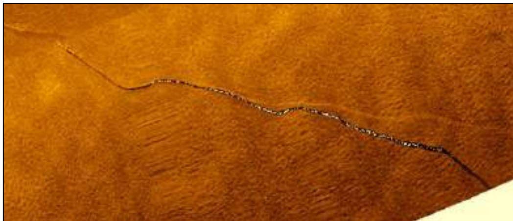
Figure 58. No measurable footprint - SSS data of mooring line #3 (NW) (09/06/21).
