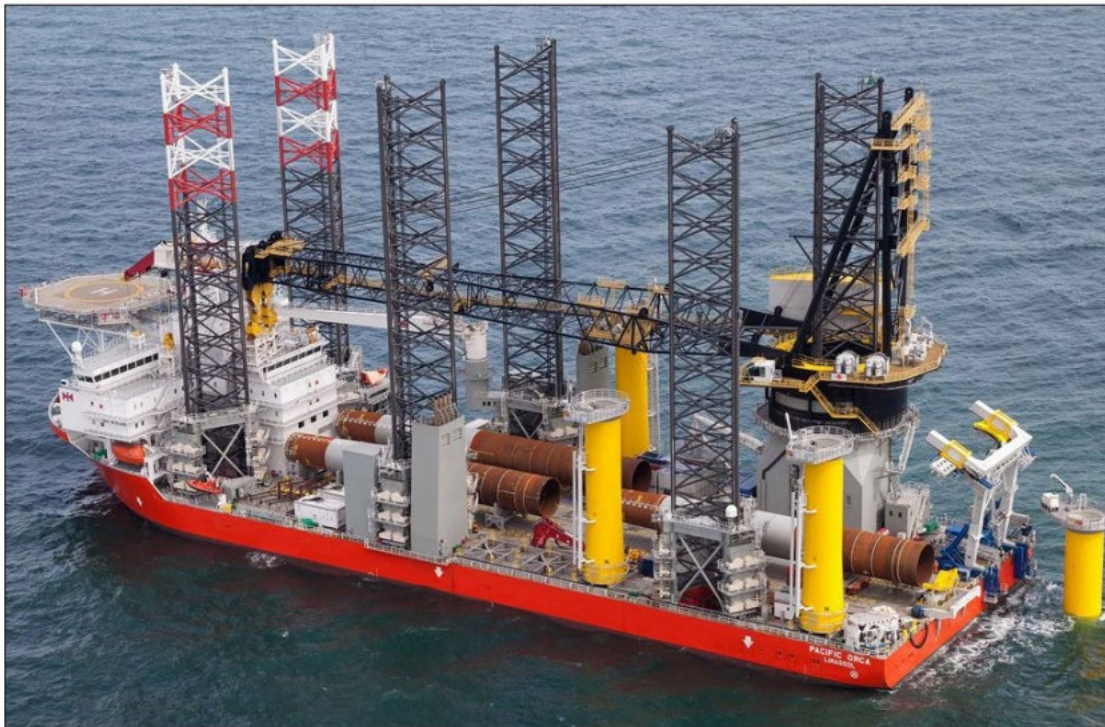
Figure 9. Monopiles on an Installation Vessel, Laying Horizontal on Deck
